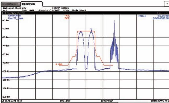
FIGURE 2 E5b testbed frequency plan
