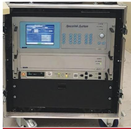
FIGURE 6 NLES E5b (NAVYS GNSS generator, L-to-C band frequency converter, Analogic filter, RF adapter)
