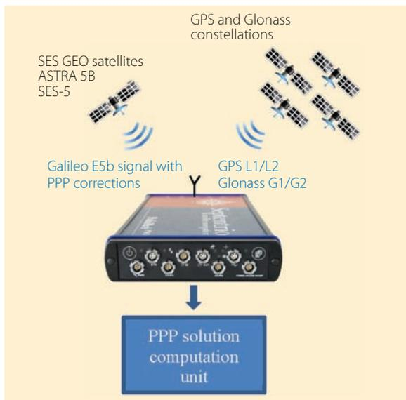
**FIGURE 7** Demonstration architecture showing the GNSS receiver used to demodulate the PPP message
