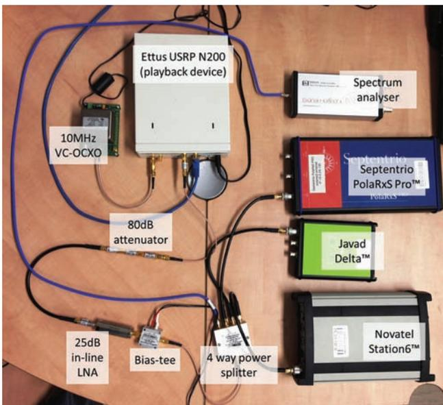
FIGURE 13 Playback equipment and test-bench configuration
