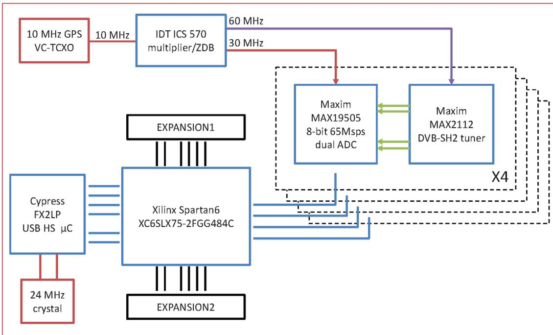
FIGURE 7 Fourtune architecture block diagram
