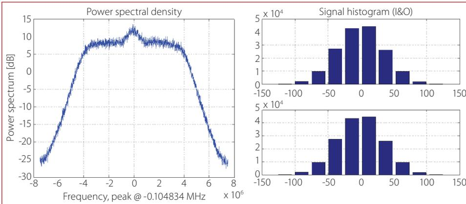
FIGURE 9 Example-spectrum and sample histogram for a single, eight-megahertz channel tuned to L1.
