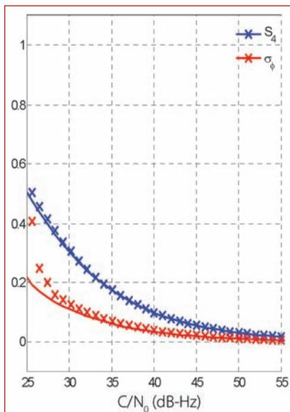
**FIGURE 6** Thermal noise contribution to the measured  $S_4$  and  $\sigma_\phi$  scintillation indices versus received carrier-to-noise-floor ratio. Solid lines represent the predicted value, as per equations (8), while the markers represent simulation measurements.
