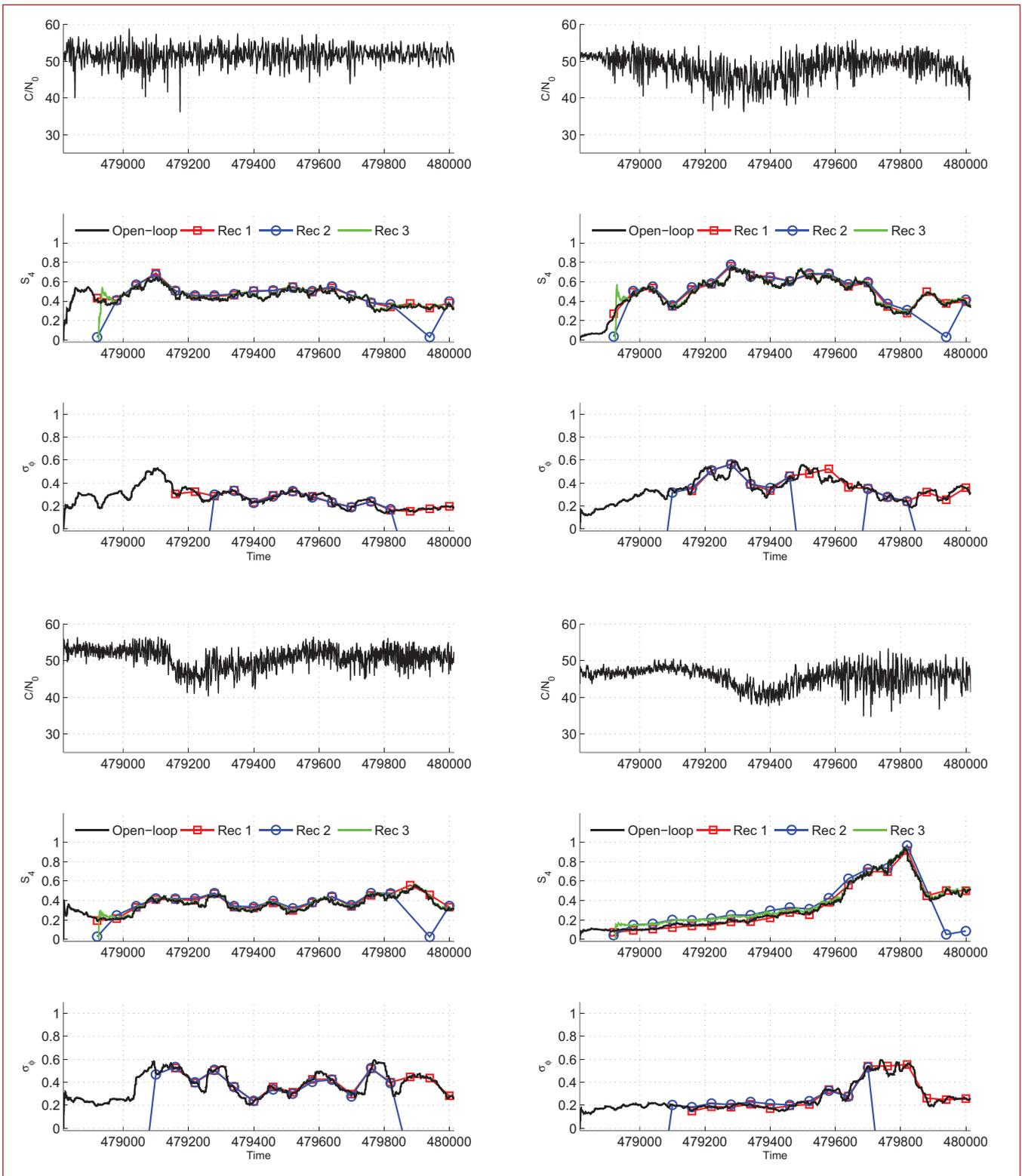
FIGURE 14 A comparison of scintillation measurements made by the new open-loop architecture and collection of commercial receivers using data collected at the Hanoi station at 13:00 UTC on the 4th of October, 2013. The loss of lock on signals is tied to zero.
