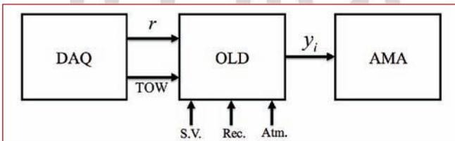
FIGURE 3 Block diagram of the open-loop receiver
