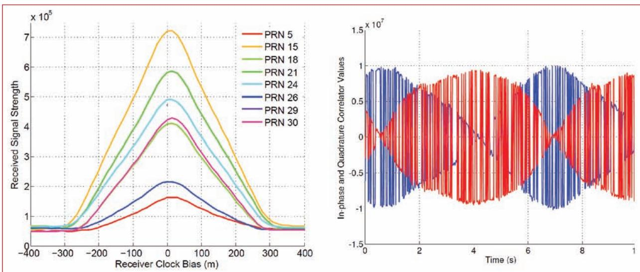
FIGURE 5 Open-loop demodulation of GPS L1 C/A signals
