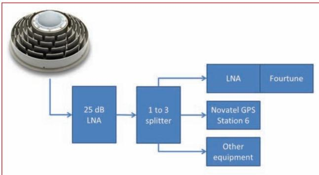
FIGURE 12 Equipment configuration at SINTEF, Norway.
