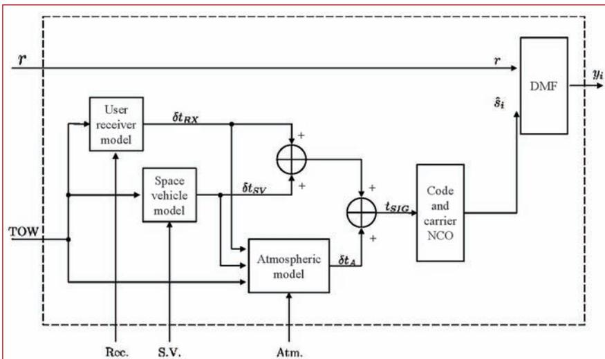
FIGURE 4 Open-loop demodulation scheme
