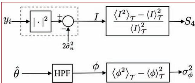
FIGURE 2 Calculation of scintillation indices from receiver variables
