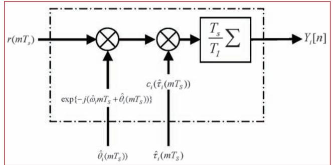
FIGURE 1 Block diagram of a digital matched filter
