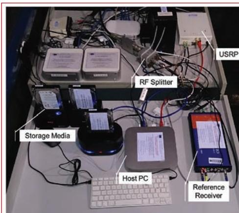
FIGURE 11 Experimental setup at the Jicamarca Radio Observatory, Lima, Peru
