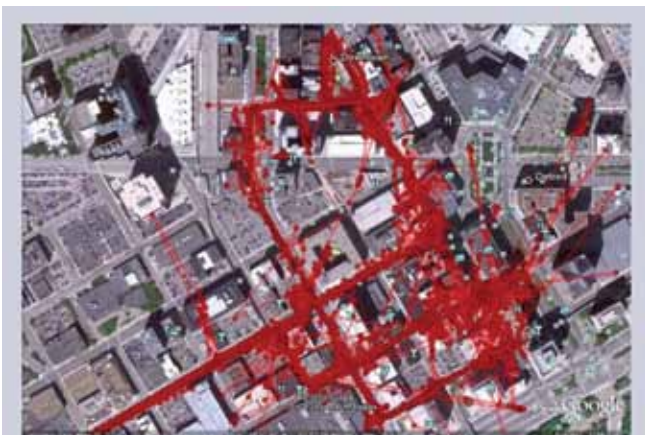
FIGURE 5 Test results for the GPS receiver with WAAS corrections for seven test trajectories
