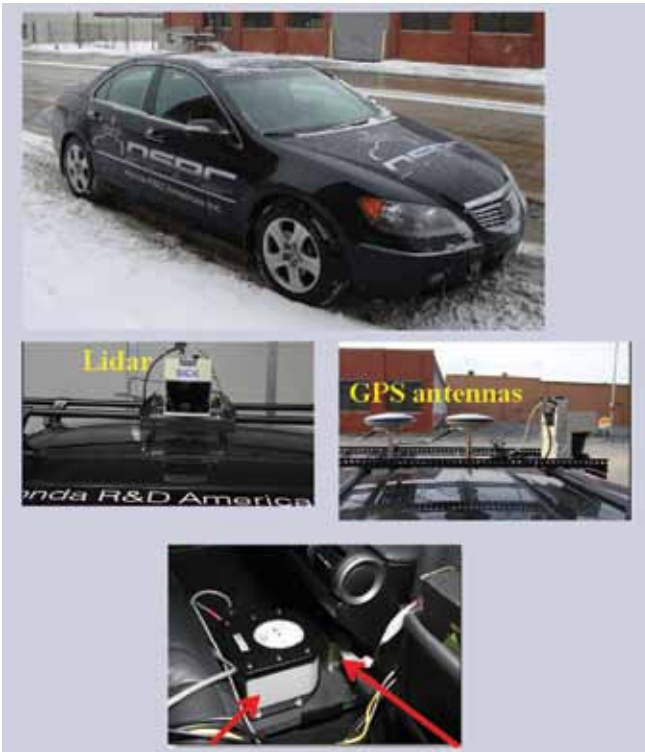
FIGURE 4 Sensor configuration for data collection on test vehicle
