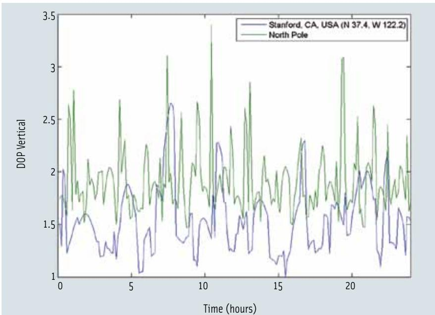
**FIGURE 9** Vertical DOP at the North Pole and Stanford, California, USA
