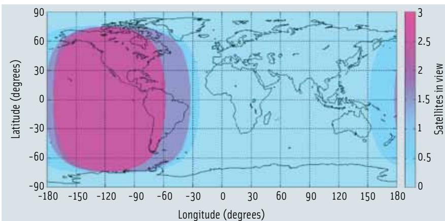
FIGURE 6 WAAS GEO satellite coverage with minimum elevation angle of 6.35 degrees. Courtesy of Tyler Reid.
