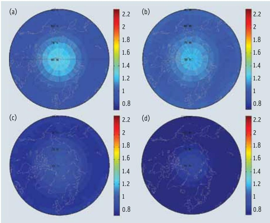
**FIGURE 10** VDOP improvement in the Arctic using two or more constellations. (a) 31 GPS + 30 Compass MEO satellites. (b) 31 GPS + 24 GLONASS satellites. (c) 31 GPS + 30 Compass + 30 Galileo satellites. (d) 31 GPS + 30 Compass + 30 Galileo + 24 GLONASS satellites.
