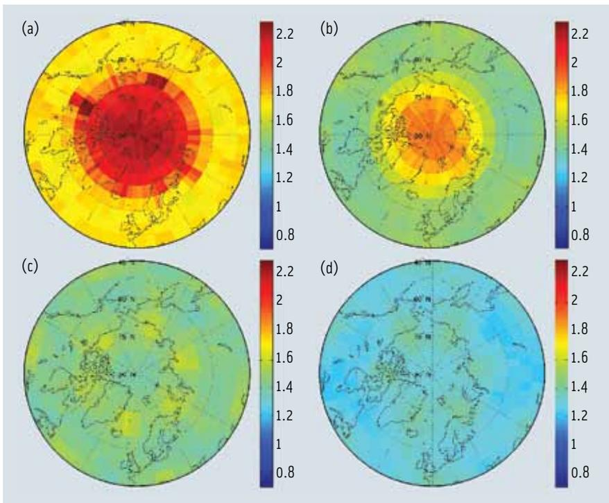
**FIGURE 8** VDOP improvement in the Arctic with the help of Iridium satellites (a). 24 GPS satellites. (b) 31 GPS satellites. (c) 24 GPS and Iridium satellites. (d) 31 GPS and Iridium satellites
