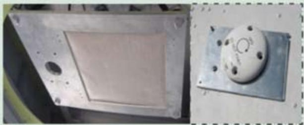
FIGURE 5 Antennas: LHCP antenna (left) and RHCP antenna (right)
