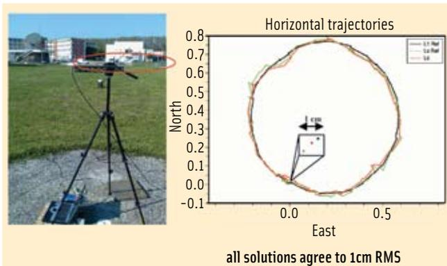
**FIGURE 1** Example of accuracy close to one centimeter provided by the integer ambiguity resolution on undifferenced phase (IARUP) technique using GPS L1 and L2 signals
