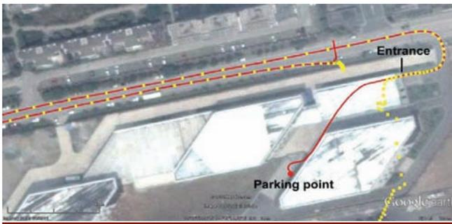
FIGURE 9 Performance of GPS/BeiDou/MEMS receiver in underground parking site
