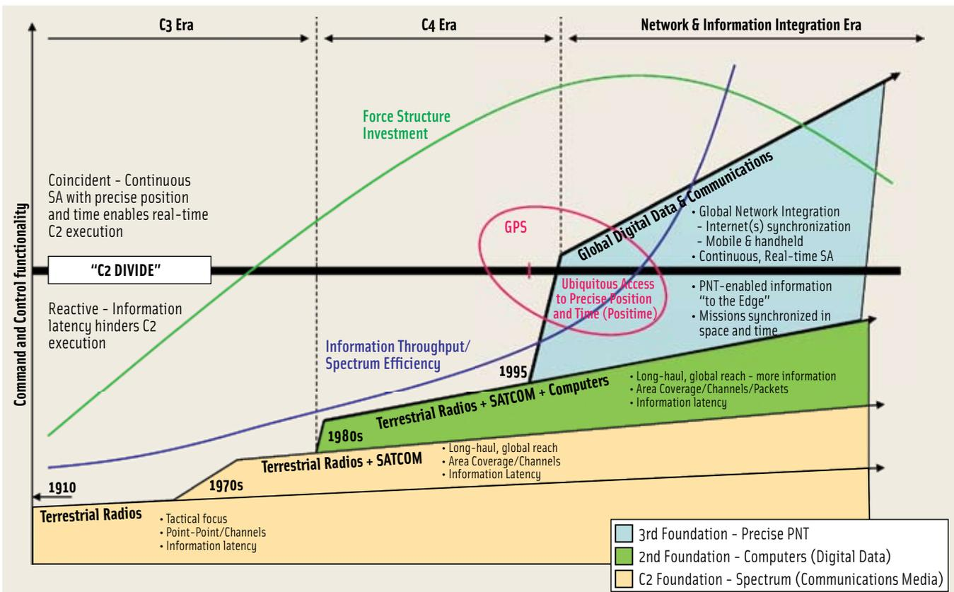
FIGURE 1 The three foundations of C2 and how they are “changing the game” in an electronic battlespace: spectrum (communications media), yellow; computers (digital data), green; PNT (precise position and timing), blue.
