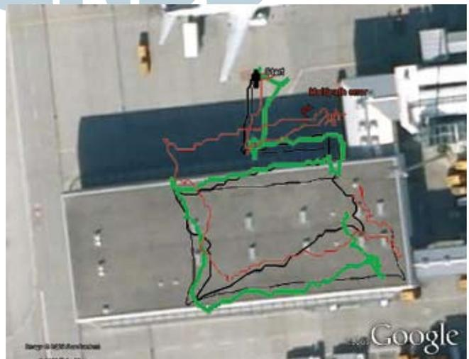
FIGURE 12 Real GPS C/A positioning results (thin black line = true trajectory, thick black line = dead reckoning, green line = ultra-tight coupled (UTC) GNSS/INS solution with two-second coherent integration time, red line = UTC solution with 35 millisecond coherent integration time and 57 non-coherent integrations)
