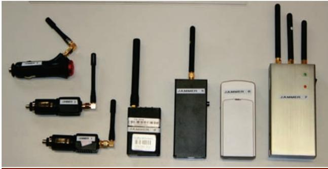
FIGURE 2 Jamming devices used for the open field measurements
