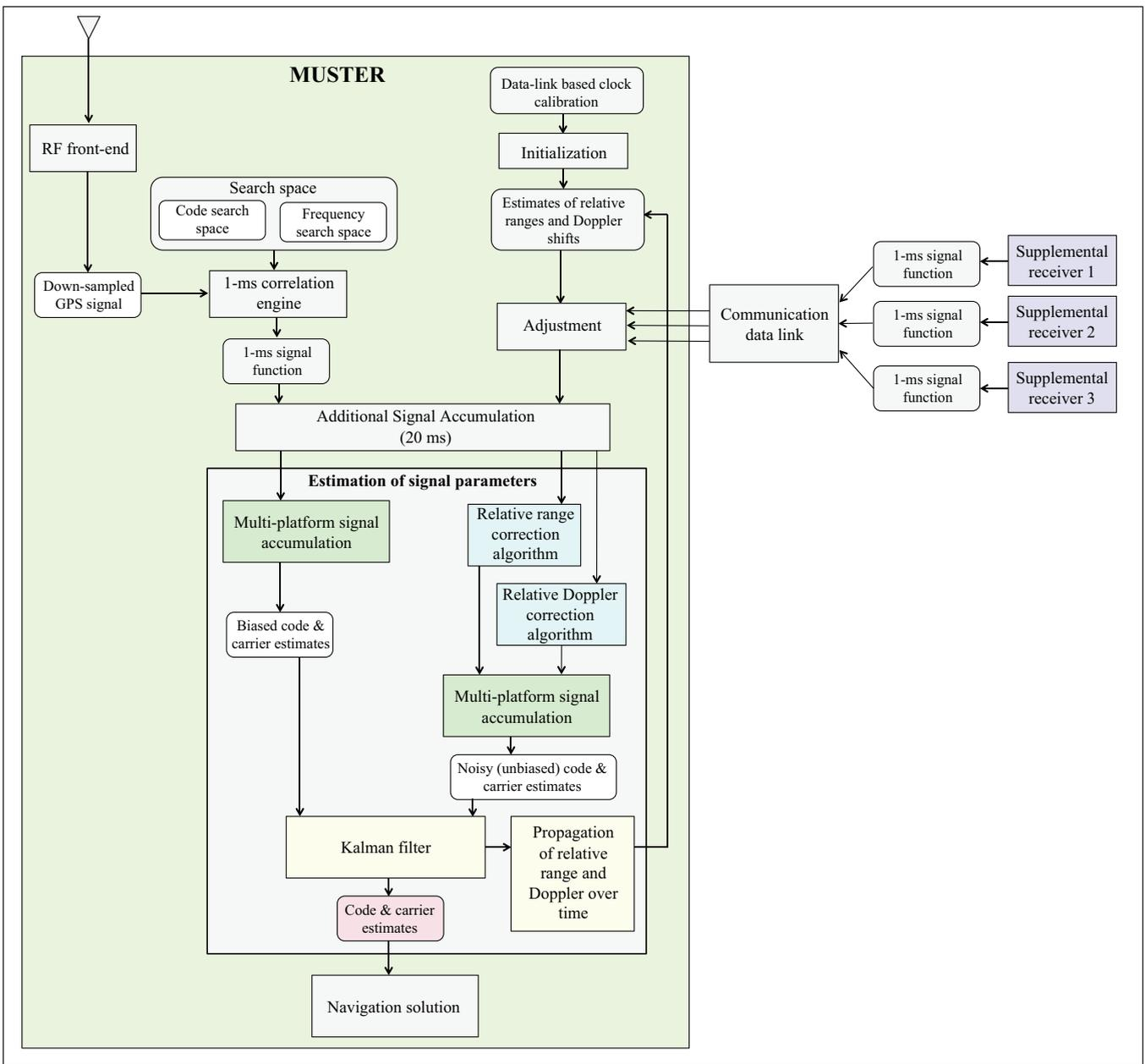
FIGURE 11 Multi-platform tracking architecture for approximately known relative navigation states.
