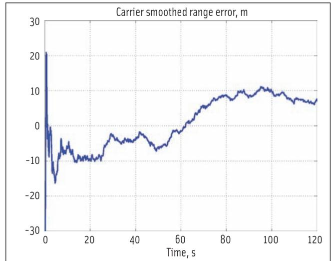
FIGURE 18 An example of MUSTER tracking results for stationary test: coherent/non-coherent signal accumulation (20-milliseconds/0.1 second integration), PRN 8 tracking, 17 dB-Hz signal
