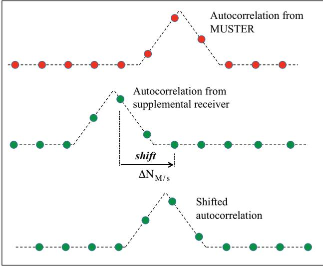
FIGURE 4 Coarse adjustment of the code autocorrelation function
