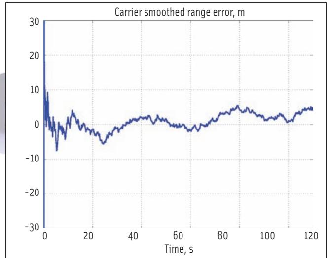
FIGURE 20 An example of MUSTER tracking results for dynamic test: coherent/non-coherent signal accumulation (20-milliseconds/0.1 second signal), PRN 8 tracking, 16 dB-Hz signal
