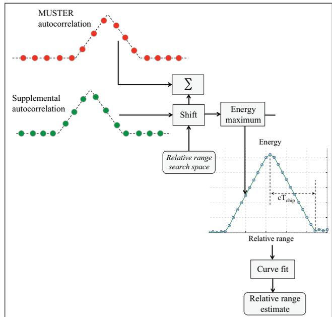
FIGURE 7 Algorithm for estimation of relative range
