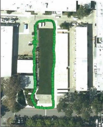
FIGURE 21 Trajectory estimation with single and multi-node signal processing in a GPS-degraded environment
