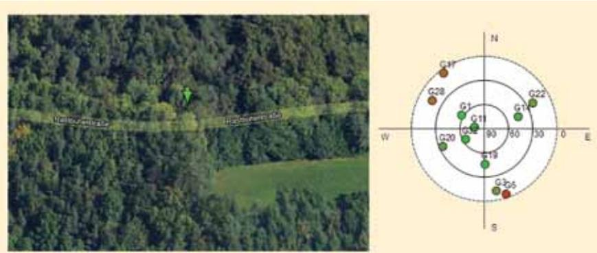
FIGURE 6 Measurement location and sky plot for the canopy test
