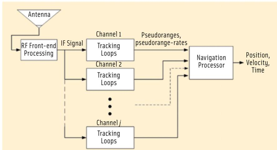
FIGURE 1 Traditional Receiver Architecture
