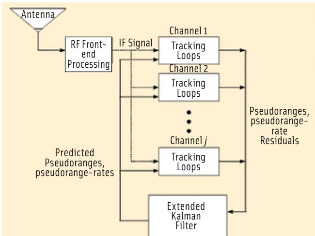
FIGURE 2 Vector Tracking Receiver Architecture
