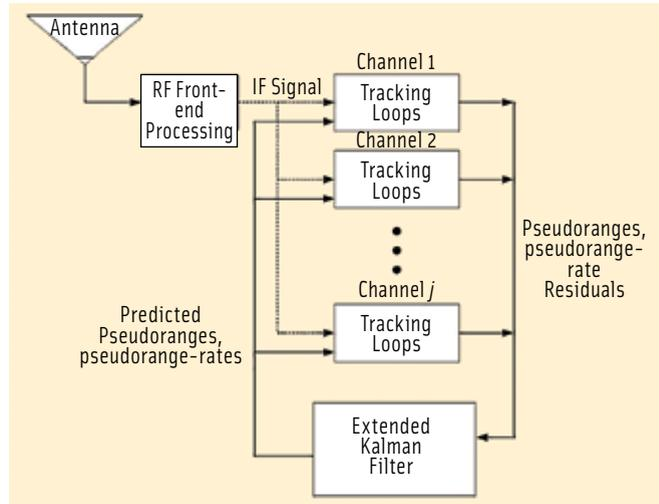
FIGURE 2 Vector Tracking Receiver Architecture
