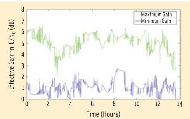
FIGURE 4 Maximum and Minimum Effective Gain from Vector Tracking
