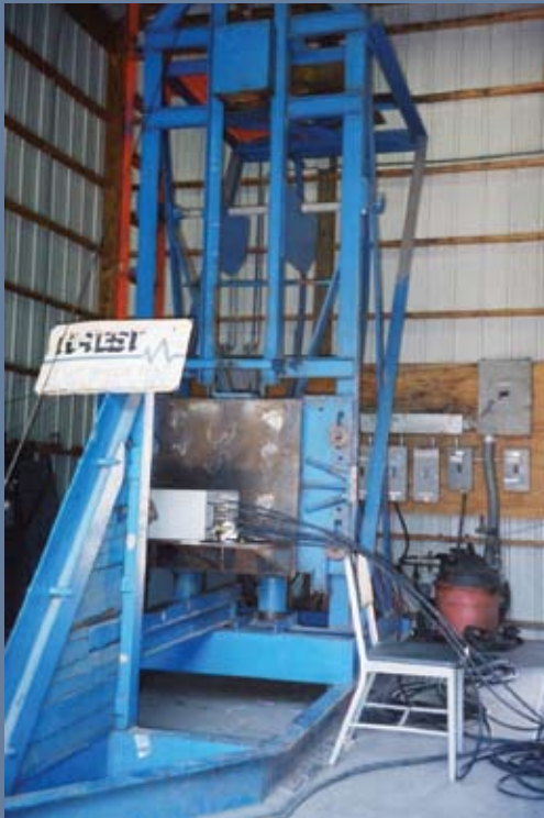
(left) SRC-40 mounted to the lightweight shock machine (above) Front panel of the SRC-40 as the hammer strikes the anvil
