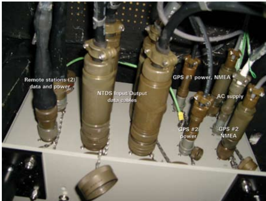
FIGURE 2 Rear panel of the Ursa Navigator with shipboard cables connected. Six cables are required for GPS data distribution. Two small cables, one for each external GPS receiver, and four large cables required for the NTDS interface.
