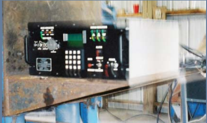
(left) SRC-40 mounted to the lightweight shock machine (above) Front panel of the SRC-40 as the hammer strikes the anvil
