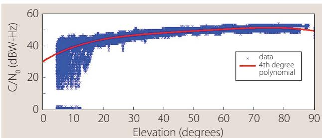
FIGURE 1 Polynomial fit of  $C/N_0$  versus elevation
