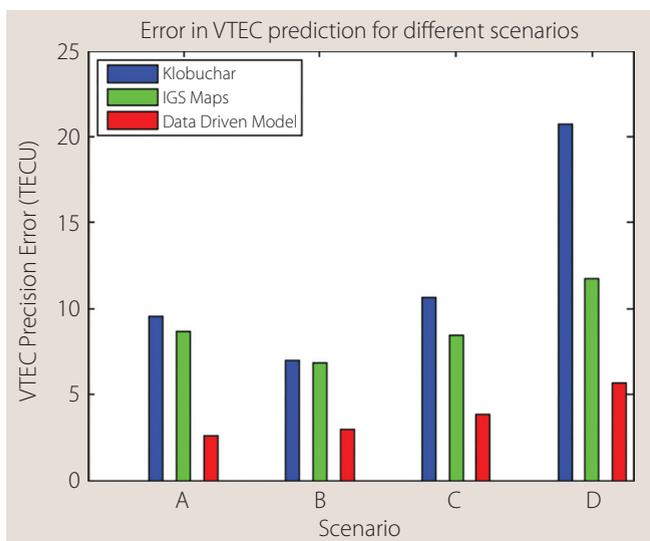
**FIGURE 3** Error in VTEC predicted by different models with respect to VTEC obtained from dual-frequency combination
