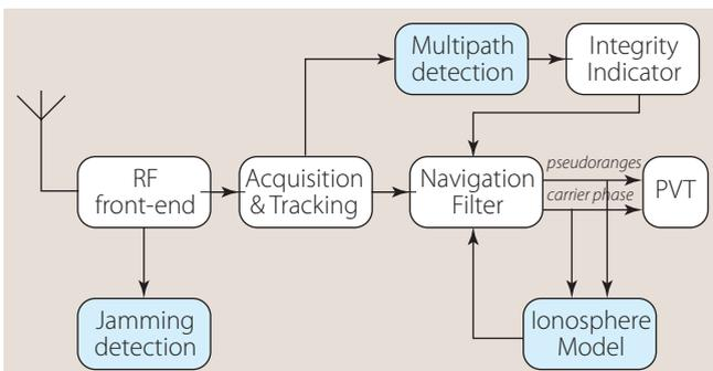
**FIGURE 5** Block diagram of the combined receiver architecture
