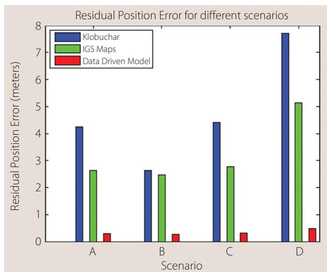
**FIGURE 4** Residual error in position when ionospheric error is corrected with VTEC predicted by different models with respect to ionospheric error mitigation (VTEC obtained from dual-frequency combination)
