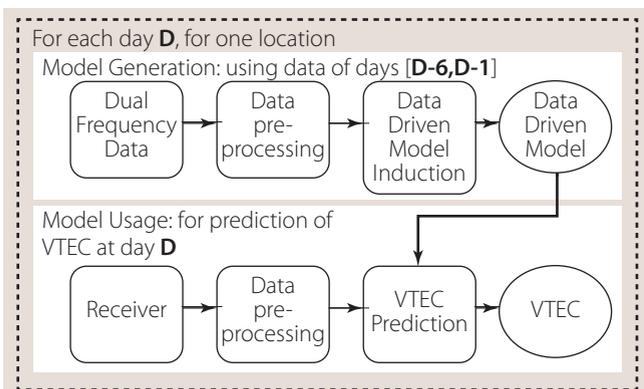
FIGURE 2 Workflow for generation and usage of data-driven ionospheric models
