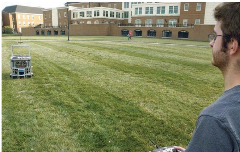
*RedBlade, operated here by Miami University senior Mark Carroll, uses multiple navigation technologies, including GNSS and Light Detection and Ranging (LIDAR).*
