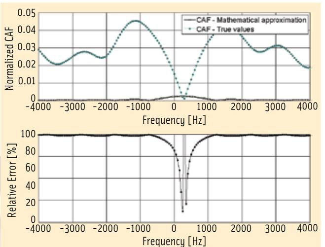
FIGURE 5 Comparison between the CAF and its mathematical approximation for a generic value of  $\Delta\tau$ , i.e.,  $\Delta\tau > 1$  chip duration (upper curve); relative error (lower curve)
