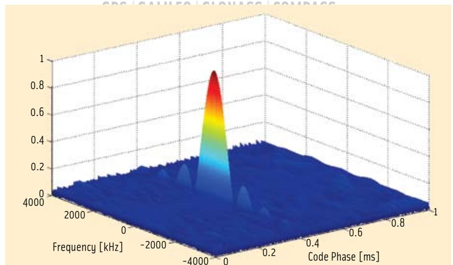
FIGURE 1 Sample of absolute value of AF in absence of noise for the L1 GPS C/A code signal
