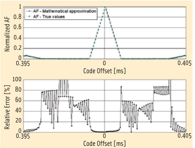
FIGURE 3 Comparison between the AF and its mathematical approximation, given by Eq. (7), for  $\bar{f}_d = f_d$  (upper curve); relative error (lower curve)
