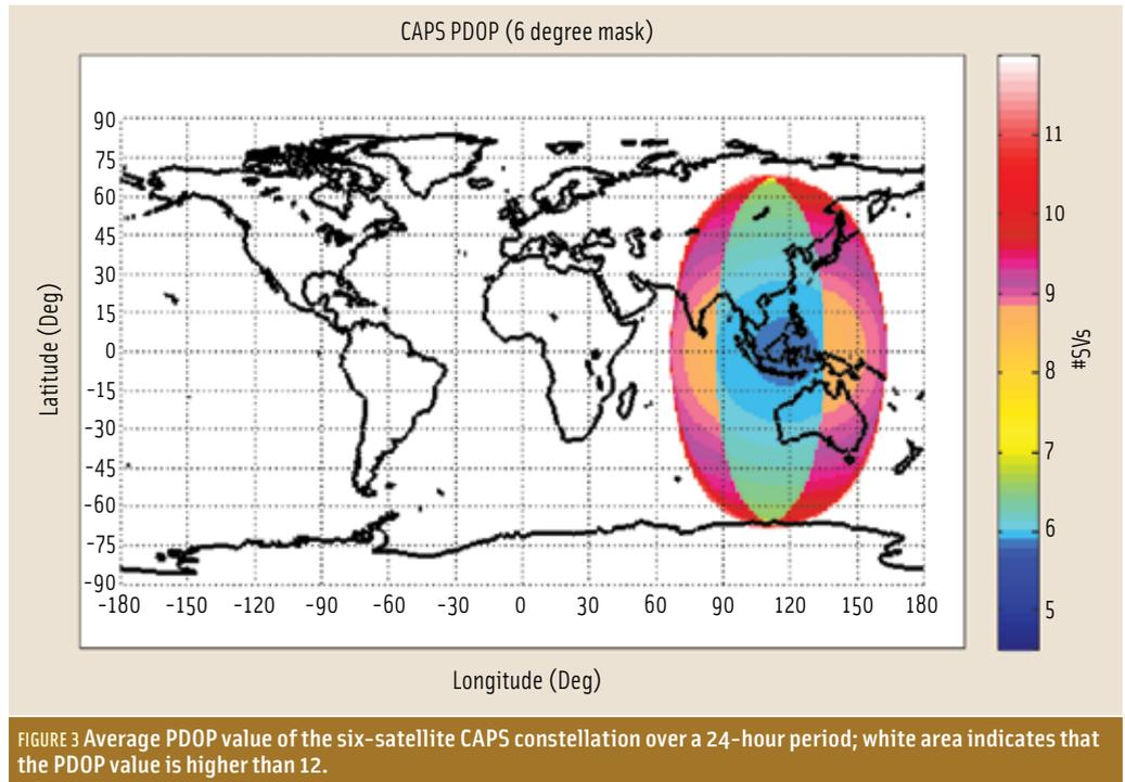
**FIGURE 3** Average PDOP value of the six-satellite CAPS constellation over a 24-hour period; white area indicates that the PDOP value is higher than 12.
