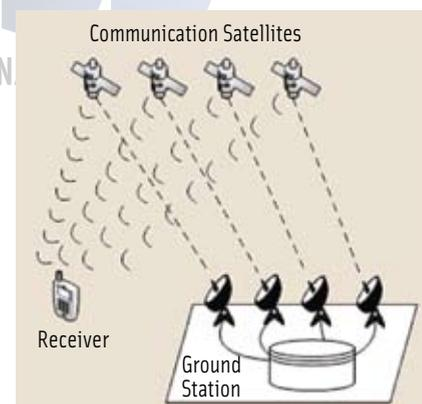
FIGURE 1 The principle of CAPS
