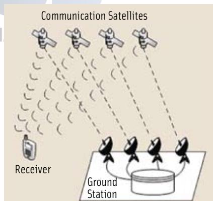
FIGURE 1 The principle of CAPS
