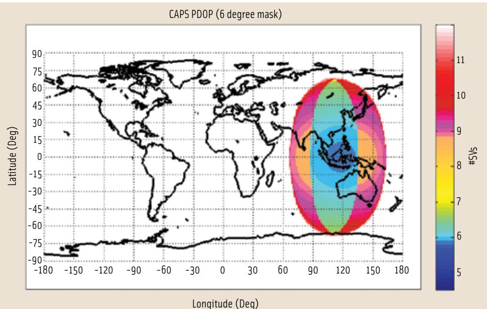
FIGURE 3 Average PDOP value of the six-satellite CAPS constellation over a 24-hour period; white area indicates that the PDOP value is higher than 12.
