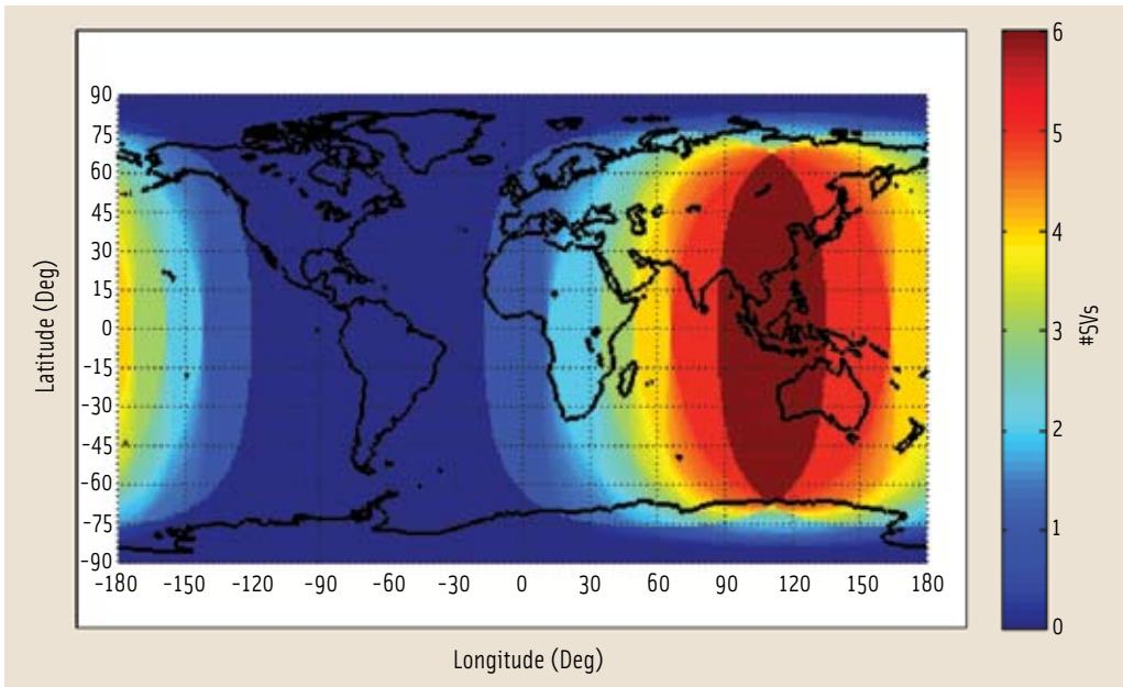
**FIGURE 2** Average number of visible satellites (above a five-degree elevation cutoff angle) of the six-satellite CAPS constellation, which consists of two GEO satellites and four SIGSO satellites with inclination of seven degrees
