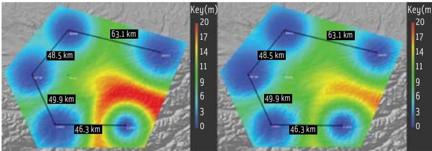
FIGURE 3 The estimated residual non-dispersive (troposphere/geometry) error for a single reference station user (left) and a network reference station user (right).
