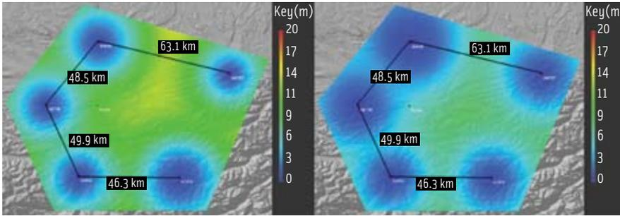
FIGURE 2 The estimated residual dispersive (ionosphere) error for a single reference station user (left) and a network reference station user (right)
