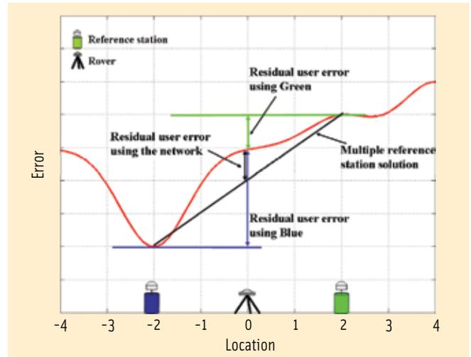
FIGURE 1 Example of the measurement error of one satellite across a region (red line). This error is measured at two locations indicated by the green and blue reference stations.
