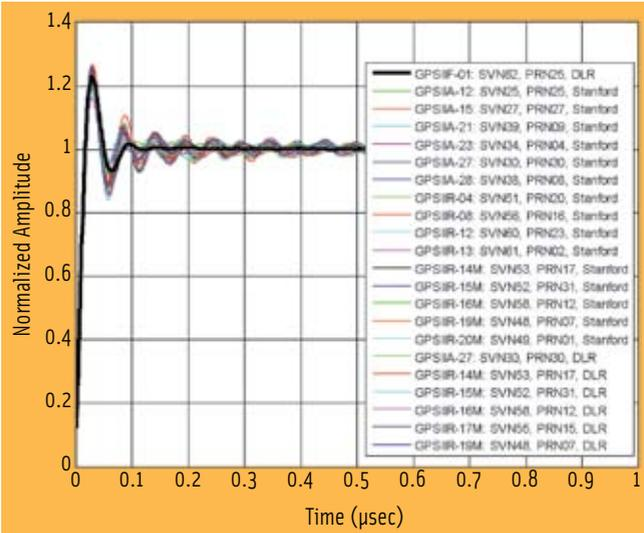
FIGURE 8 Comparison of the step responses on the L1 C/A codes of 17 GPS satellites. The response of SVN62 is depicted by the heavy black trace.
