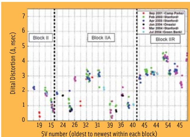
FIGURE 6 Historical digital distortion plotted as a function of SVN, from earliest to latest launch date (from A. Mitelman)
