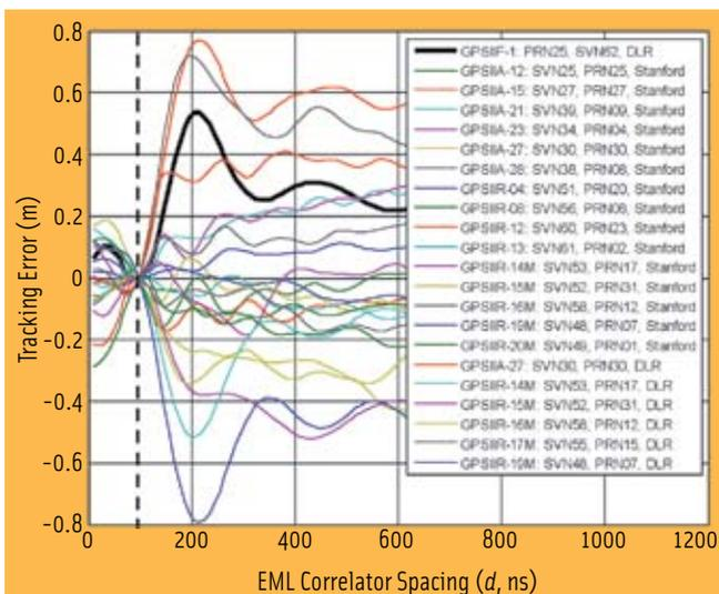
FIGURE 11 Tracking errors of all satellites relative to mean across all satellites plotted as a function of Early-Minus-Late (EML) correlator spacing,  $d$ .
