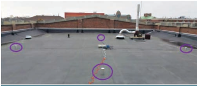
FIGURE 5 Four antennas located on roof of Talbot Laboratory, University of Illinois at Urbana-Champaign. Reference image of the setup taken from the article by D. Chou et alia listed in Additional Resources.
