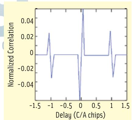
**FIGURE 3** Correlation pattern for the Strobe correlator with 200 ns delay spacing
