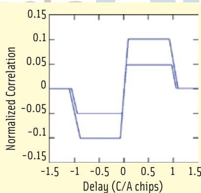
**FIGURE 2** Narrow correlators 100ns and 200ns delay spacing
