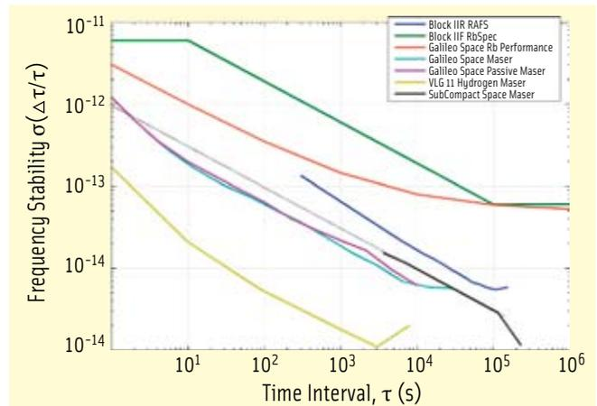
FIGURE 2 Stabilities of the various clocks used in GPS or yet to be used in Galileo. All except the specification lines are based on data taken at NRL or published for Galileo.
