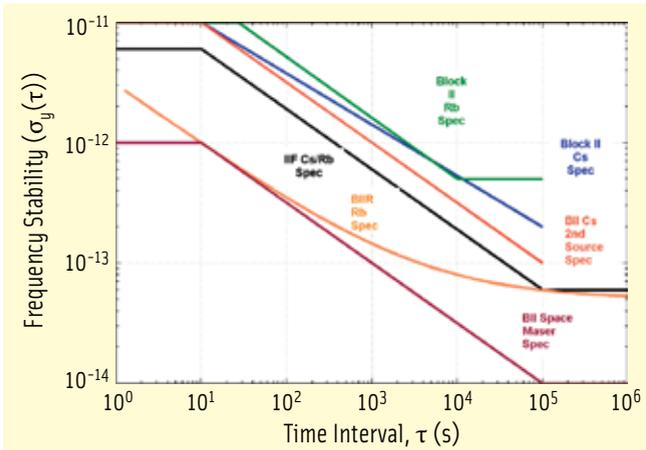
FIGURE 1 Space clock stability specifications for GPS. They are expressed in terms of frequency stability ( $\sigma_y(\tau)$ ), which represents the time error accumulating as a function of the interval after update.
