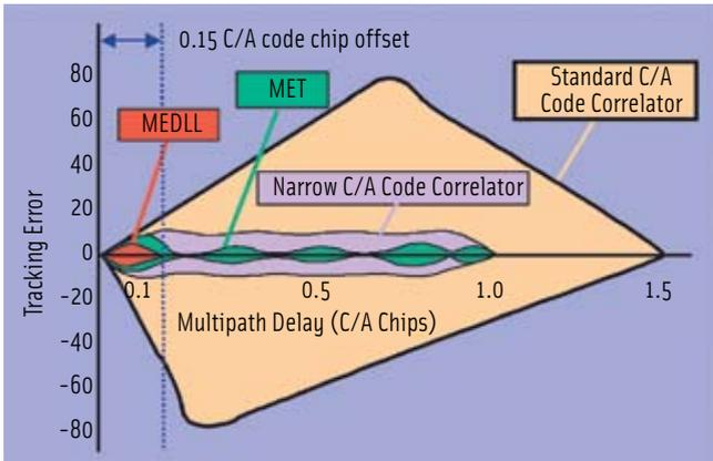
**FIGURE 1** Different pseudorange multipath mitigation schemes, including narrow and standard code correlators, Multipath Elimination Technique (MET), and Multipath Estimation Delay Lock Loop (MEDLL)
