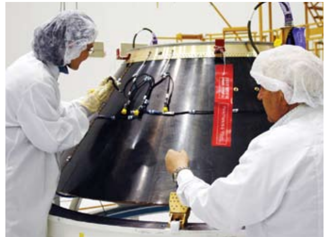
Preparing the adapter between Soyuz and Giove-A
