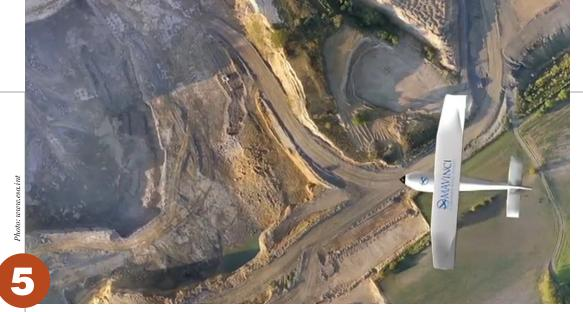
MAVinci autonomous micro air-vehicle surveys an open mining site.
