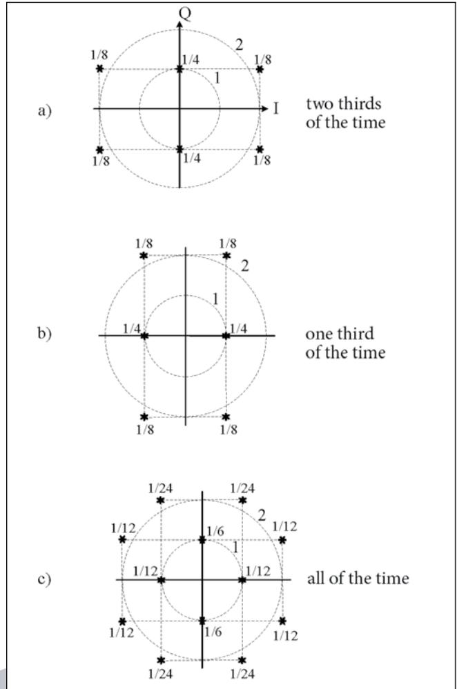
FIGURE 8 Phase diagram of symmetrized three-component sum
