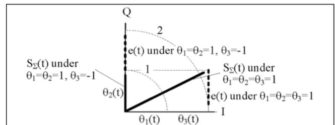
FIGURE 1 Summary signal  $S_{\Sigma}(t)$  vectors alignment by interplex modulation for the case  $\theta_1 = \theta_2 = 1$ ,  $\theta_3 = \pm 1$
