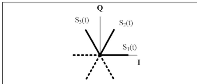
FIGURE 3 Vector diagram of three-component symmetrical MSPM
