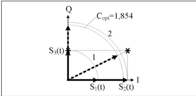
FIGURE 7 Phase diagram of three-component aligned sum
