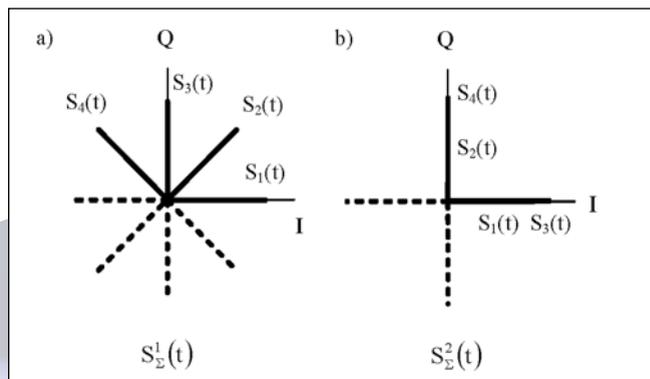
FIGURE 5 Vector diagrams of four-component symmetrical MSPM
