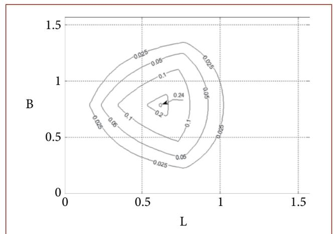
FIGURE 2 Dependence LCA from B and L for interplex modulation
