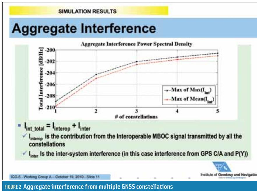
**FIGURE 2** Aggregate interference from multiple GNSS constellations
