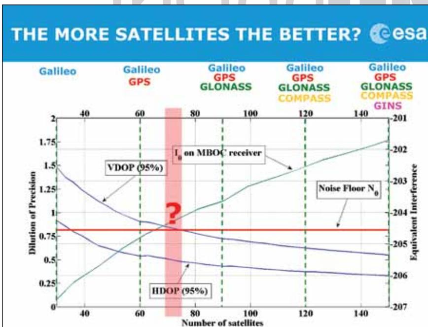
FIGURE 1 Satellite geometry, signal availability, and noise
