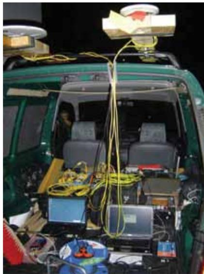
*Equipment installation inside the test vehicle*
