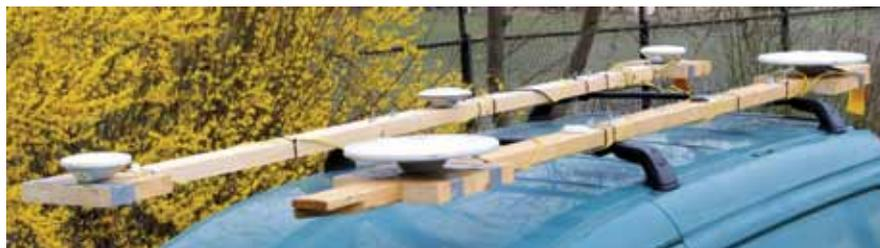
*Antenna set-up on the roof of the test vehicle*
