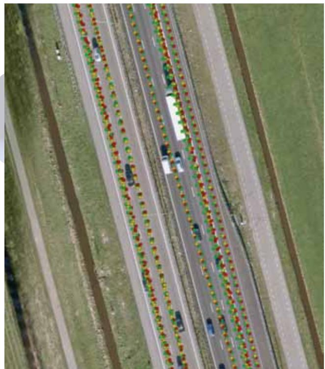
FIGURE 3 SF-PPP position trajectories from one session of the field trials overlaid on an aerial image. This figure demonstrates a lane change to the inside lane on the left side of the northbound traffic. Green dots represent positions determined by the low-end GPS receiver, red dots for the mid-range receiver, and yellow for the high-end receiver. The trajectories correctly indicate the lanes in which the vehicle was traveling at the time.
