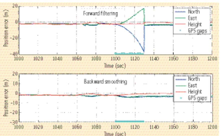
FIGURE 10 Comparison of Forward Filtering and Backward Smoothing Position Drift during a GPS Signal Outage
