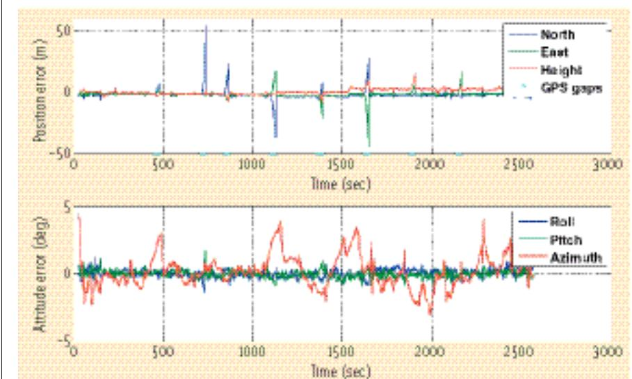
FIGURE 5 Navigation Errors of the MEMS inertial system during 30-second GPS signal outages
