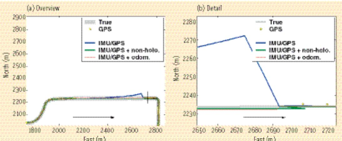
FIGURE 8 A typical case showing the effect of non-holonomic constraint and odometer update during GPS signal outages
