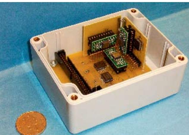
FIGURE 3 System using MEMS IMU sensors
