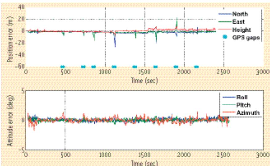
FIGURE 6 Navigation Errors of the MEMS inertial system during 30-second GPS signal outages (with non-holonomic constraint)
