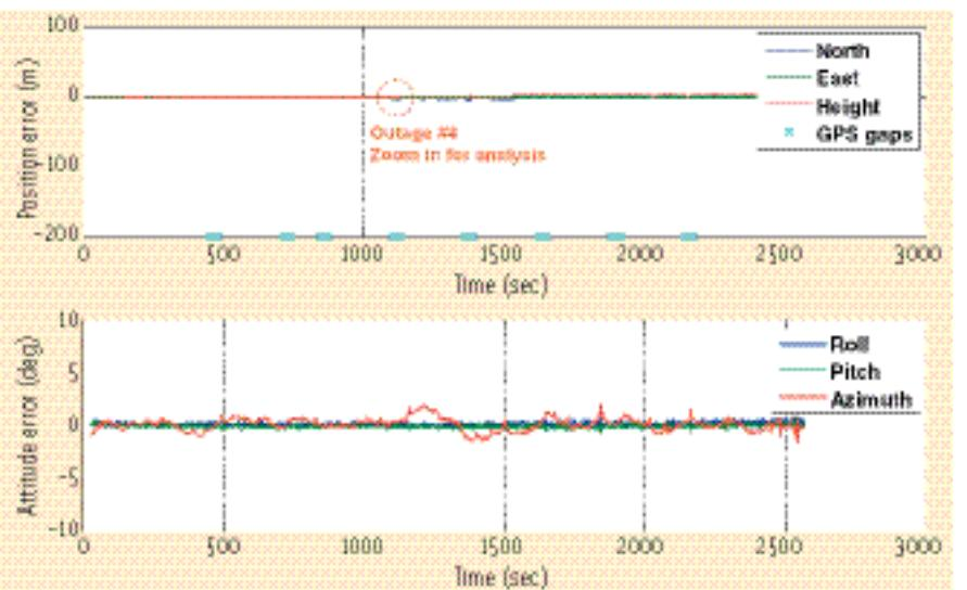
FIGURE 9 Backward smoothing errors of the MEMS inertial system during 30-second GPS signal outages
