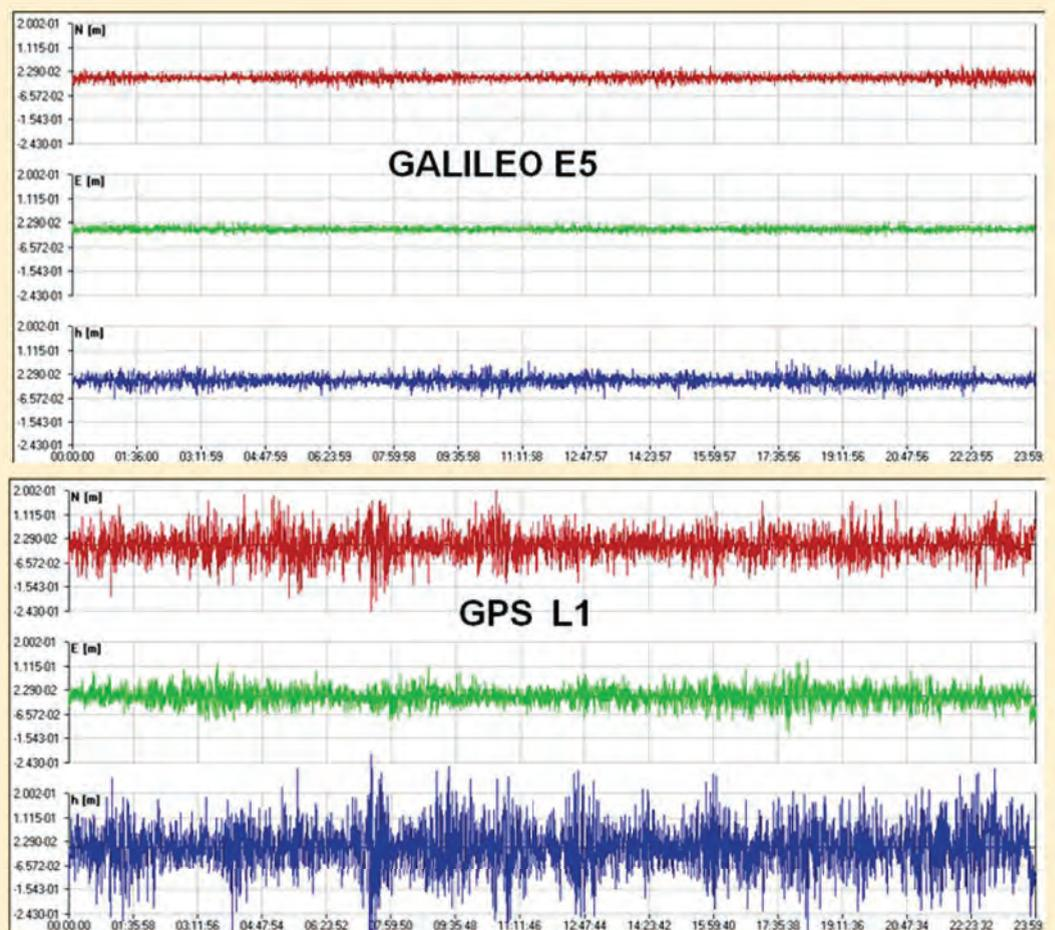
FIGURE 5 Comparison of the time series of the three coordinate components using simulated Galileo E5 (upper plot) and GPS L1 (lower plot) CPC results; 2.290-02 is read 2.290·10<sup>-2</sup> meters; GNSS time of day format is hh:mm:ss
