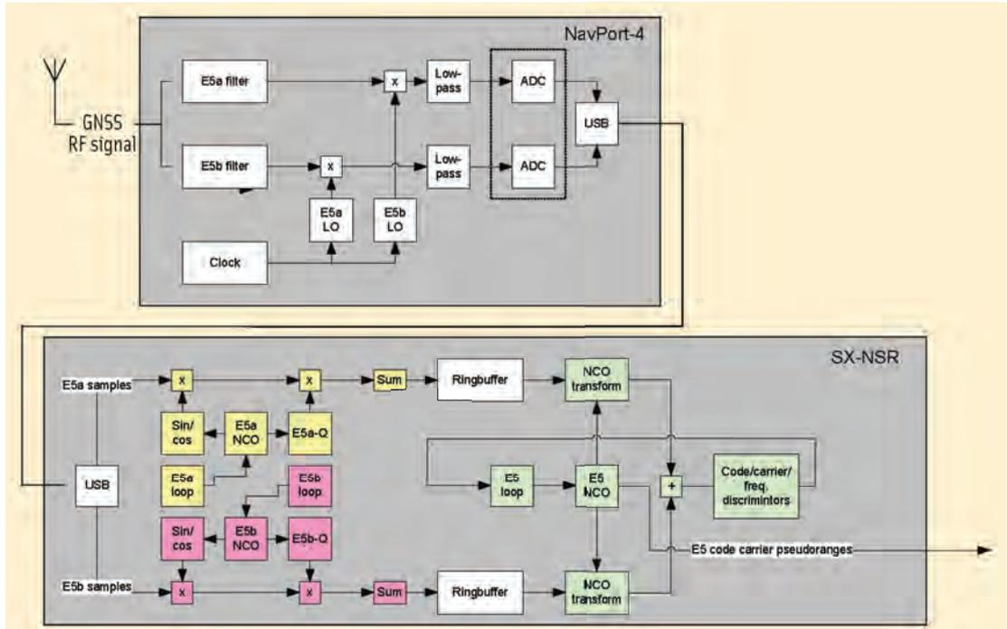
FIGURE 2 Software-defined receiver implementation
