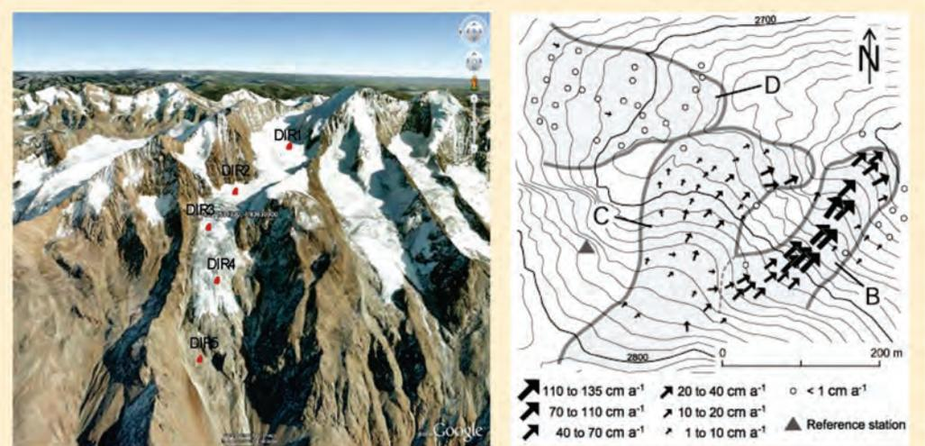
FIGURE 6 Observation network on the Dirru rock glacier (left, courtesy of Google Maps) and a velocity map of the glacier (right) [data from C. Lambiel and R. Delaloye, cited in Additional Resources]
