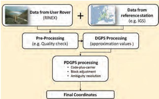
FIGURE 4 Processing procedures of Galileo E5 single-frequency data
