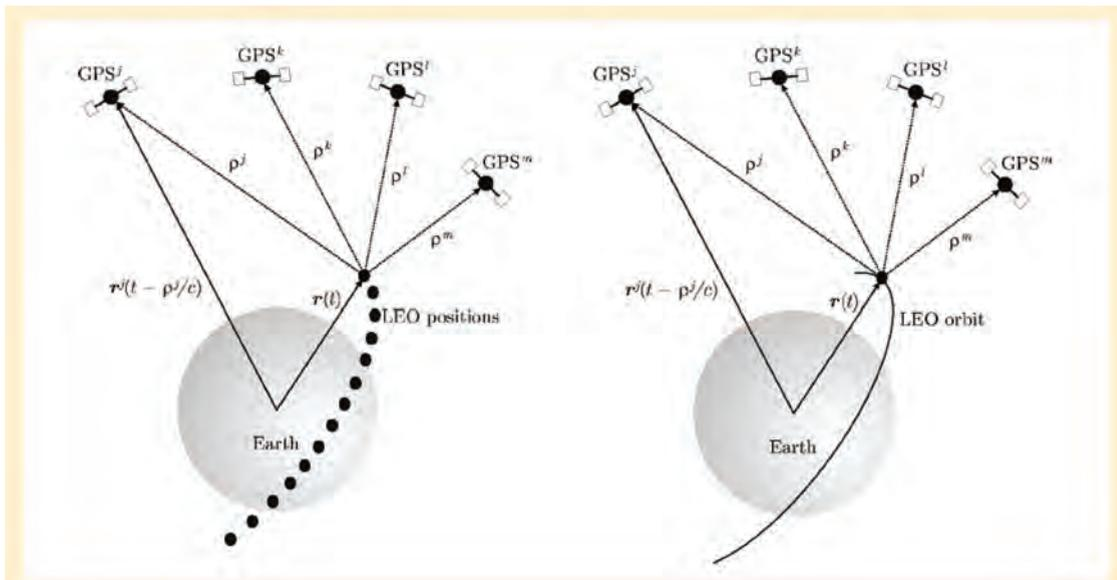
**FIGURE 12** Kinematic (left) and reduced-dynamic (right) orbit generation for a LEO
