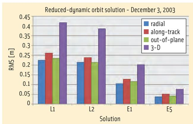
**FIGURE 13** Reduced-dynamic orbit solutions: RMS values (meters) of differences to ENVISAT reference orbit, December 3, 2003
