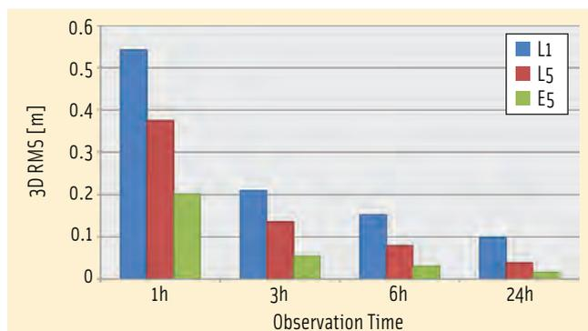
**FIGURE 9** Comparison of the 3D RMS error of different time series using Galileo E5, GPS L1 and GPS L5 CPC results
