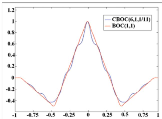
**FIGURE 11** Normalized autocorrelation functions computed over  $\pm 15$  MHz bandwidth
