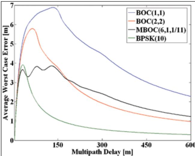
FIGURE 15 Average error for noncoherent early-late processing (NELP), BW=14 MHz (Ideal Brickwall filter), d=0.05 chips
