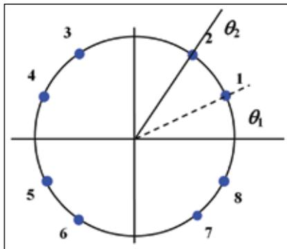
**FIGURE 10** Modified 8-PSK modulation with constant envelope for the optimized signal
