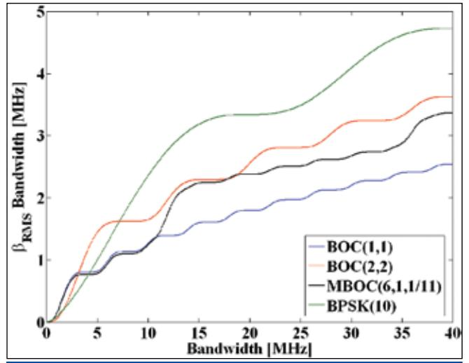
FIGURE 16 RMS bandwidth vs. two-sided receiver bandwidth (Ideal Brick-wall filter)
