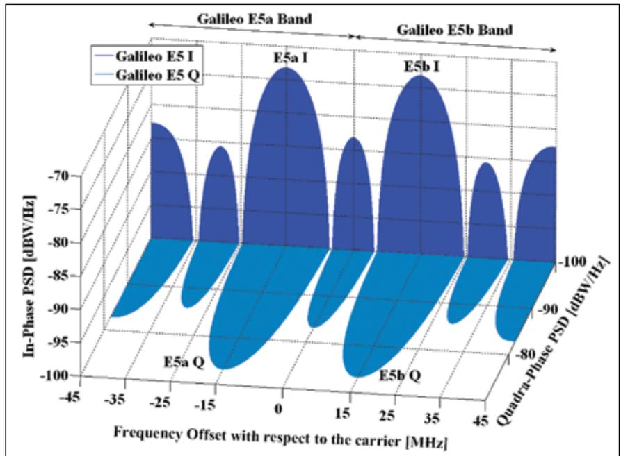
**FIGURE 4** Spectra of Galileo Signals in E5 [4]
