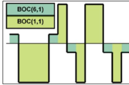
**FIGURE 7** Pseudo-random time multiplexing of BOC(6,1) and BOC(1,1) in the CBOC solution
