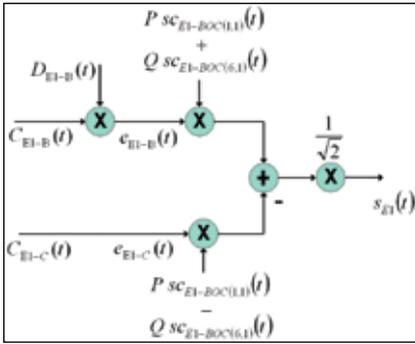
**FIGURE 6** Modulation scheme of Galileo E1 signals
