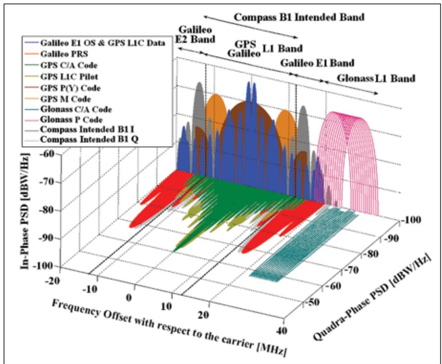
FIGURE 1 Spectra of GPS, Galileo, GLONASS and Compass Intended Signals in E1/L1
