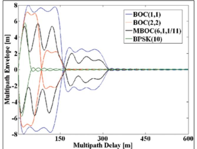
FIGURE 14 Multipath Error Envelope for noncoherent early-late processing (NELP), BW=14 MHz (Ideal filter), d=0.05 chips
