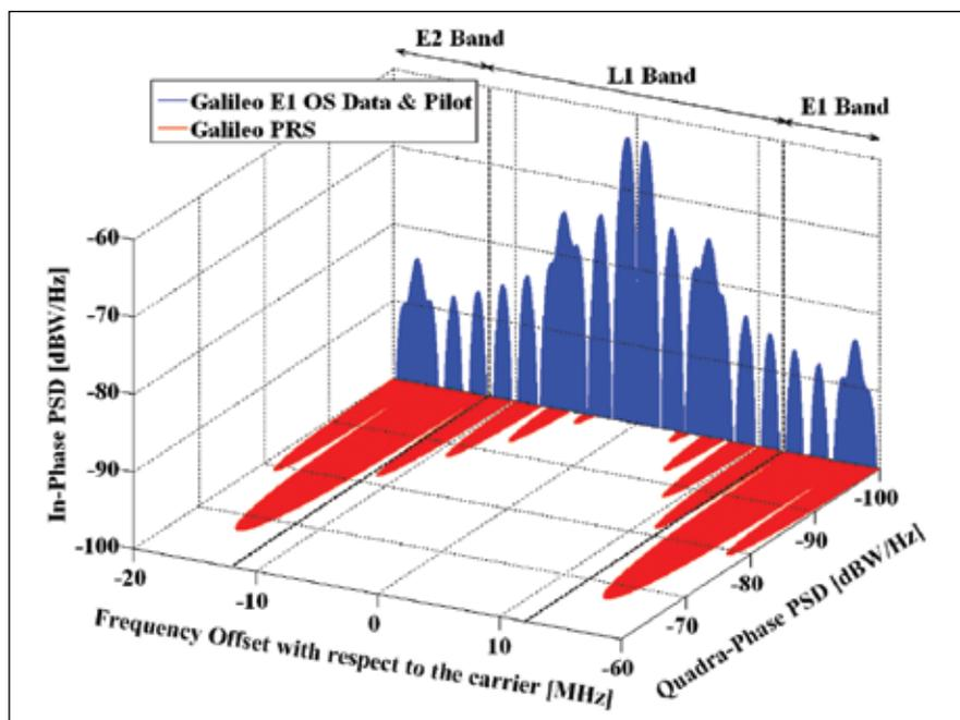
**FIGURE 12** Spectra of Galileo Signals in E1
