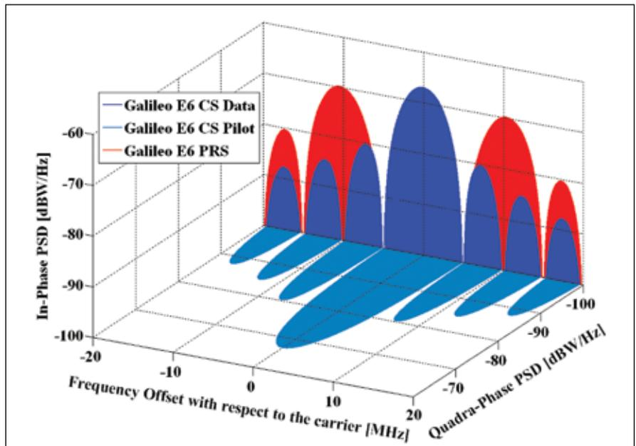
**FIGURE 5** Spectra of Galileo Signals in E6
