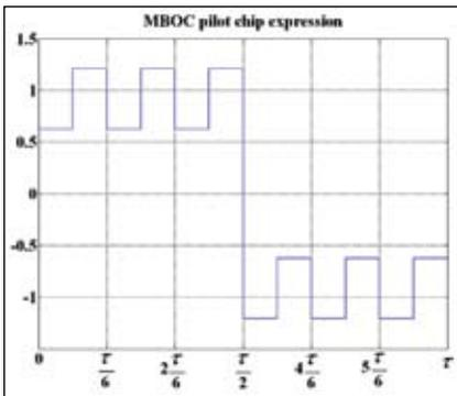
**FIGURE 9** Pilot CBOC pilot chip with BOC(1,1) and BOC(6,1) in anti-phase
