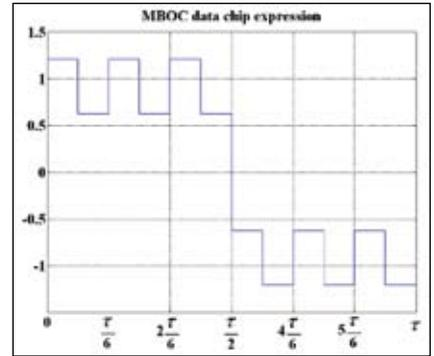
**FIGURE 8** Data CBOC data chip with BOC(1,1) and BOC(6,1) in-phase
