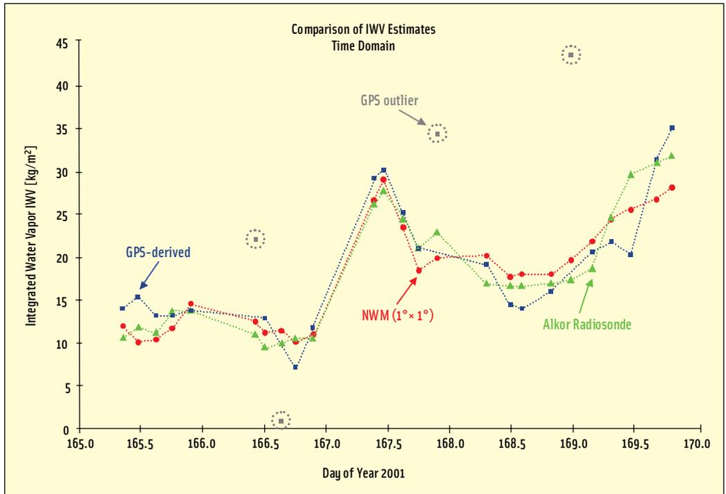
FIGURE 2 Comparison of GPS-, radiosonde and weather-model (NWM) derived water vapor samples during the Alkor experiment.
