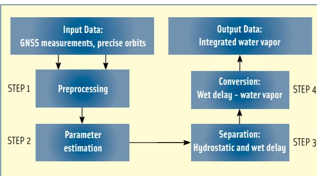
**FIGURE 1** Processing chain for GNSS-based integrated water vapor determination.
