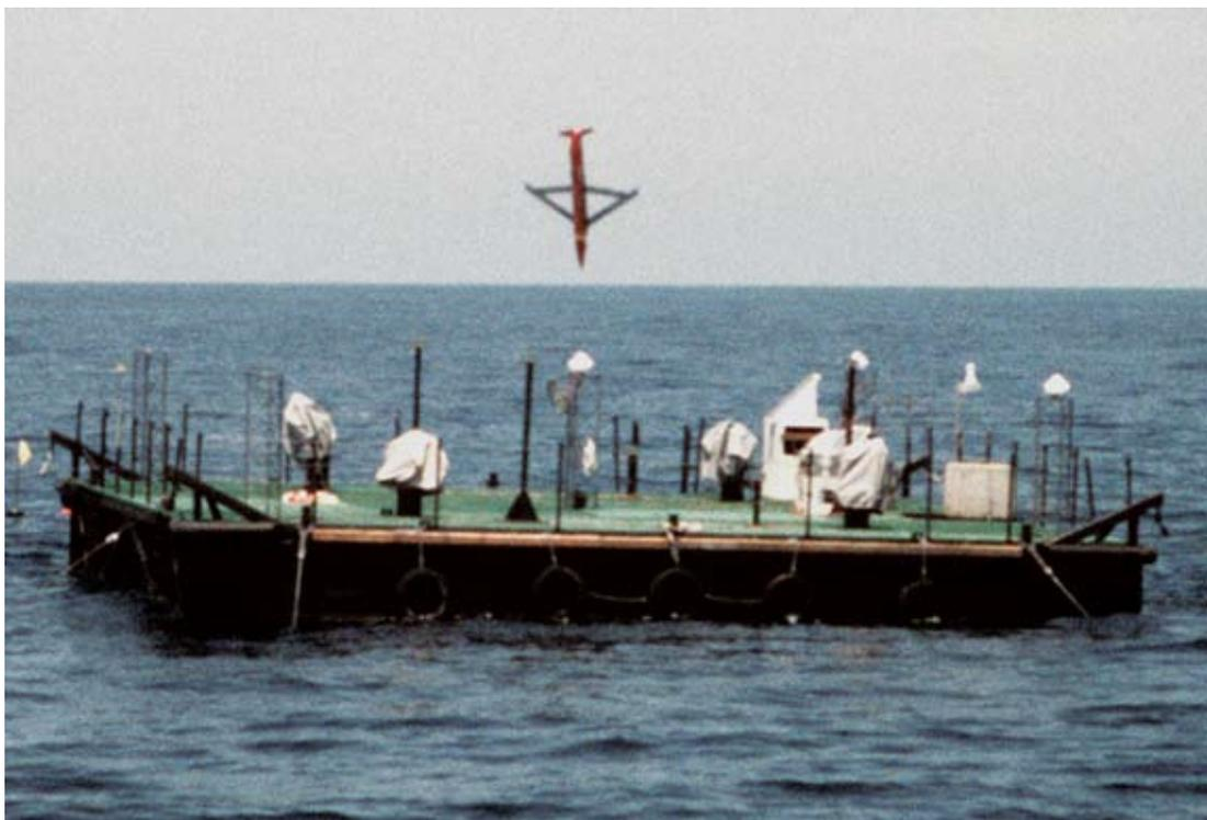
A Small Diameter Bomb (SDB), one of the Air Force's premier new weapons, is pictured just prior to impact against one of the OTTA floating targets. The SDB is a 250-pound class GPS precision guided glide bomb capable of penetrating 13 feet into a target from 70 miles away.
