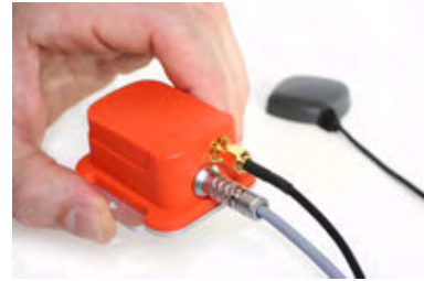
Figure 2: MEMS-based MTi-G Miniature AHRS
