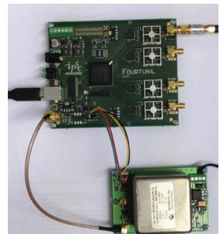
FIGURE 8 Fourtune front-end and GNSS-disciplined reference oscillator
