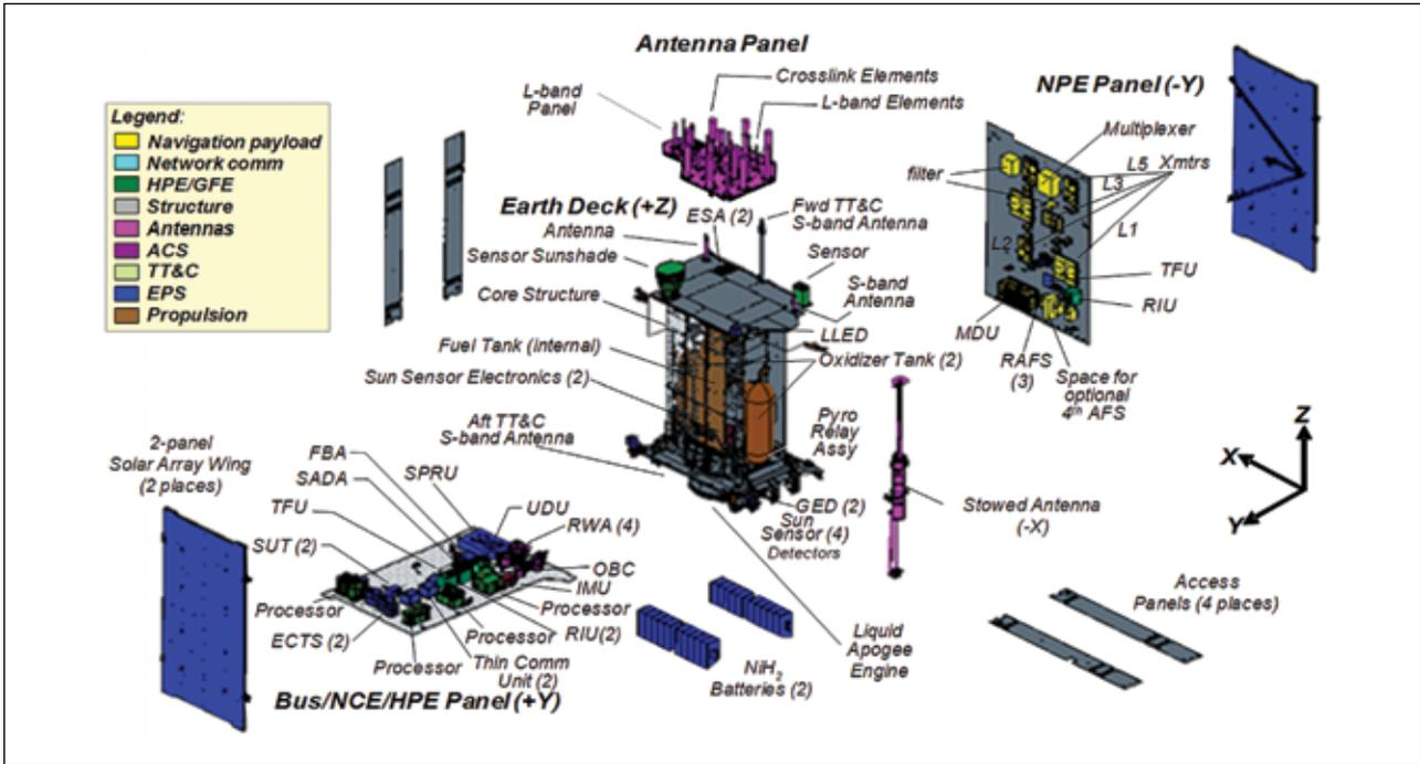
FIGURE 4 GPS III expanded view
