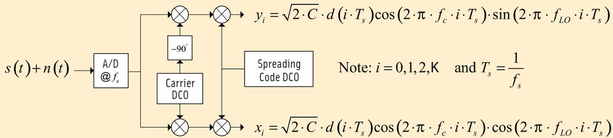
FIGURE 2 Carrier power estimation (spreading code synchronized)
