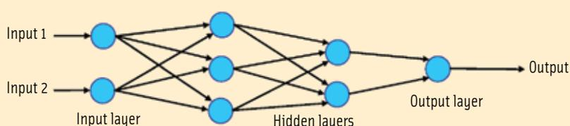
FIGURE 1 Multi-layer feed-forward neural network
