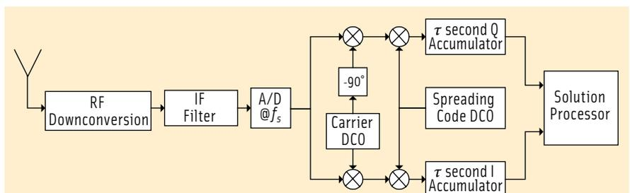
FIGURE 1 Typical GNSS receiver block diagram
