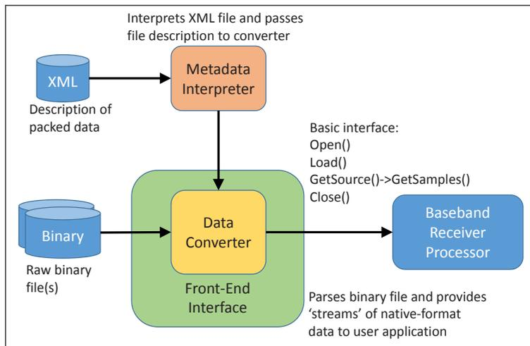
FIGURE 6 Example of the Normative Reference Software configured as a software GNSS receiver front-end
