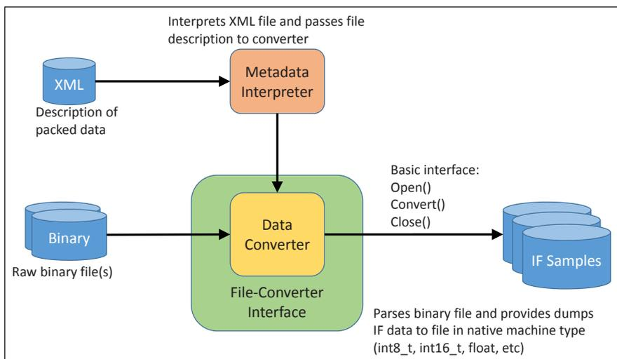
FIGURE 5 Example of the Normative Reference Software configured as a file converter
