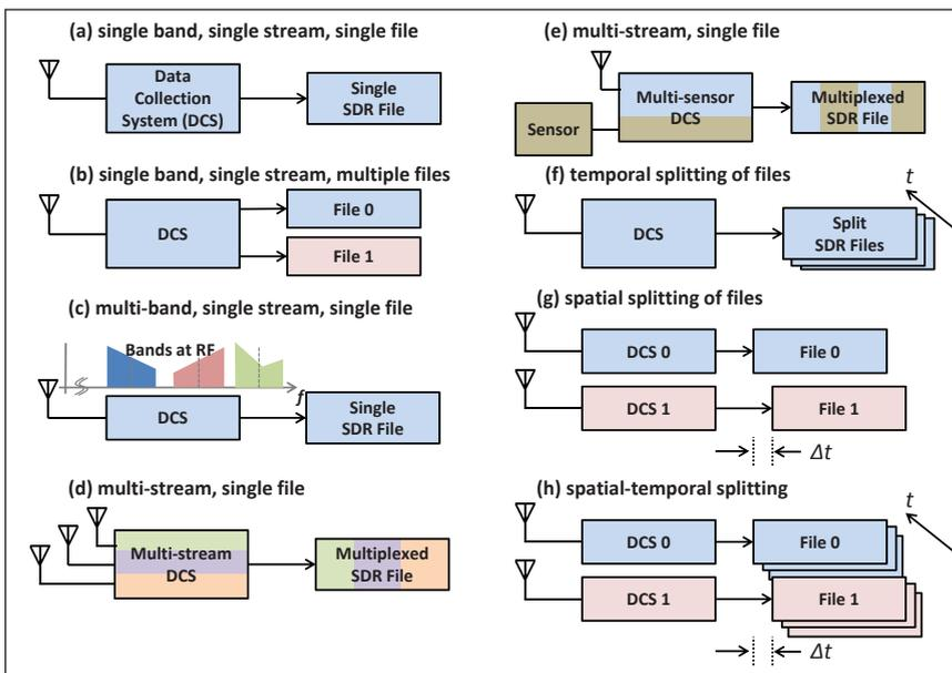
FIGURE 3 Fundamental GNSS SDR Data Collection Topologies
