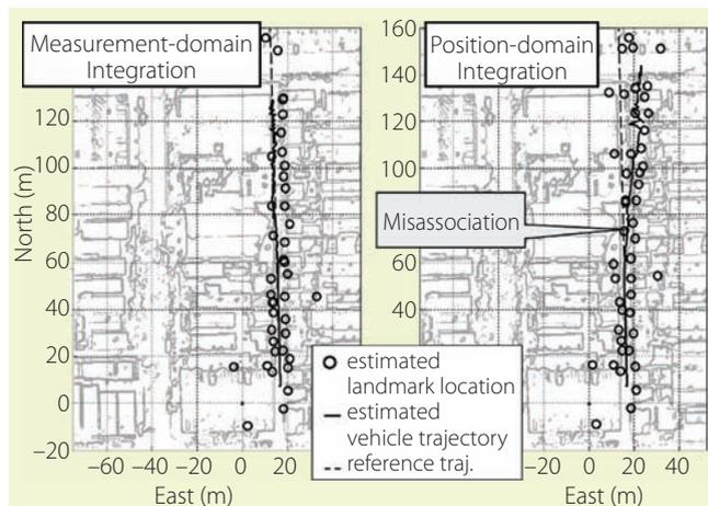
**FIGURE 6** Impact of Incorrect Association on Vehicle Trajectory Estimation. The position-domain integration scheme on the right-hand side experiences a missed association when the measurement-integration scheme on the left-hand side does not. In this case, the left-hand side can be considered truth reference trajectory; because of the missed association, the flawed estimated right-hand side trajectory indicates that the vehicle drove into multiple building walls.
