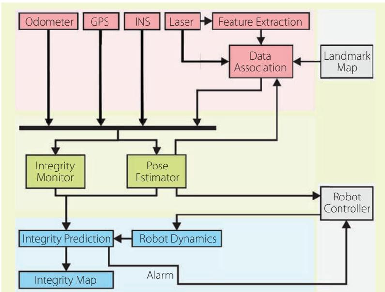
**FIGURE 5** Example HAV Navigation System. Key Sensors are represented on top. Their measurements are processed to estimate HAV position, velocity and orientation, and then to predict safety risk and send alerts if needed.
