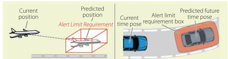
**FIGURE 4** Safety Risk Prediction Concept. To ensure safety, the predicted vehicle position must be within a predefined acceptable limit called the “alert limit” (AL) box. Integrity is the probability of the vehicle being inside the box while accounting for both nominal sensor errors and faults. The AL box is an order of magnitude smaller for HAV than it is for aircraft applications.
