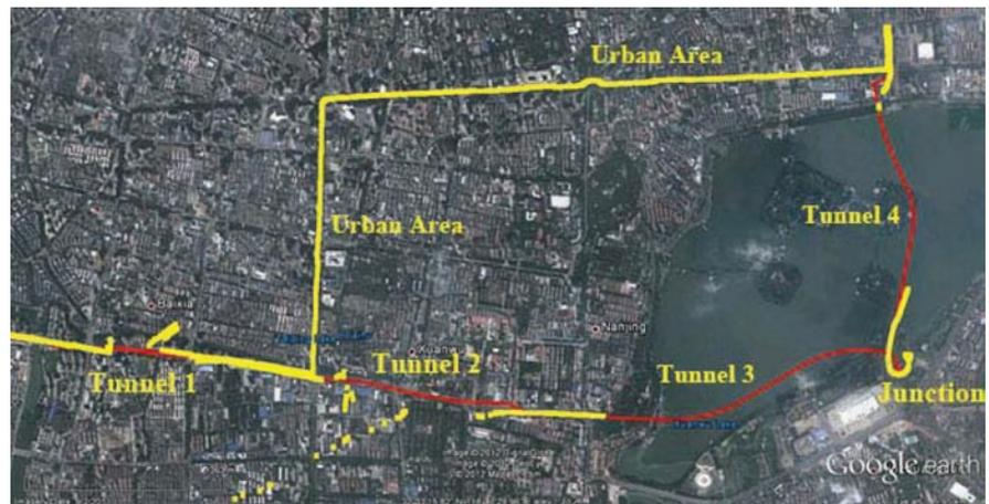
FIGURE 5 Two-way road test in Nanjing: yellow, GPS/BeiDou positioning; red, GPS/BeiDou/MEMS positioning
