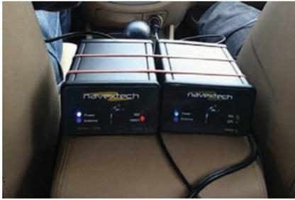
GPS/BeiDou/MEMS configuration (left) and GPS/MEMS configuration (right)
