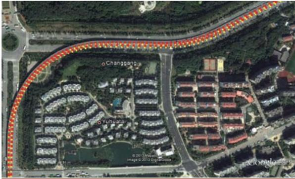
**FIGURE 7** Solutions from GPS-only (red) and GPS/BeiDou (yellow) on airport highway
