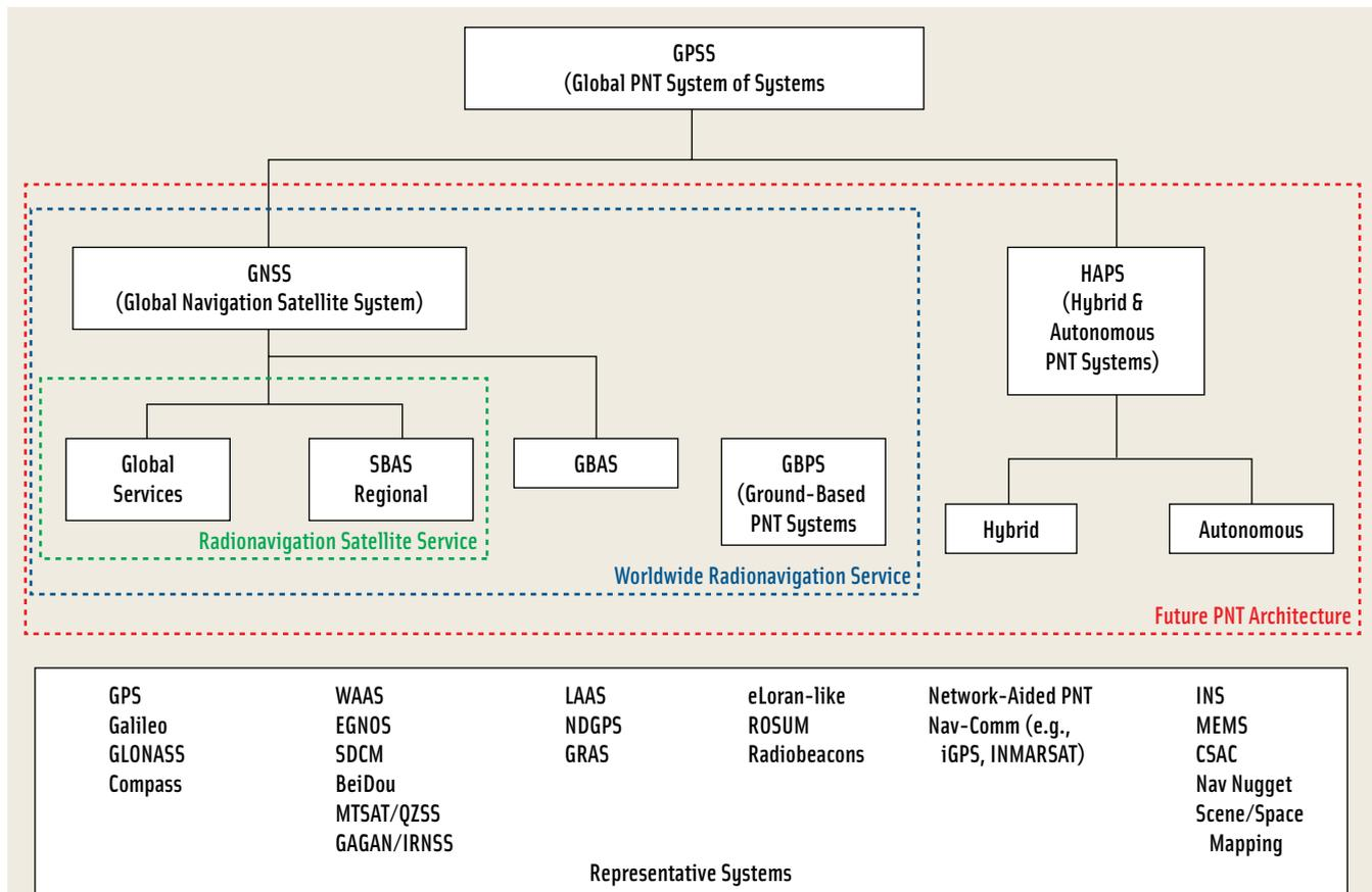
FIGURE 2 The Global PNT System-of-Systems
