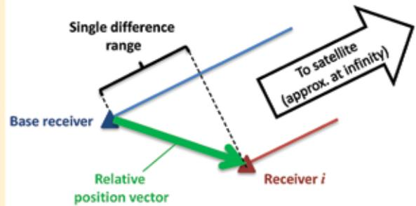
**FIGURE 1** Illustration relating single difference measurements to the relative position vector between two points. The single difference measurement is essentially the projection of the relative position vector onto the line of sight vector to the satellite.
