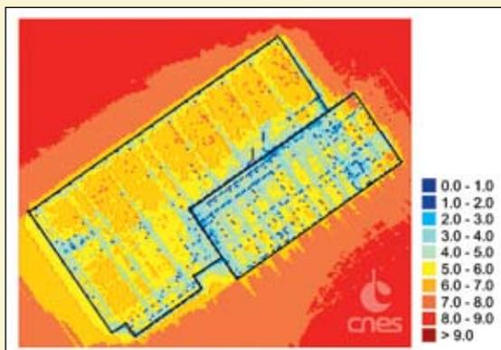
FIGURE 5 Average number of available A-Galileo signals in acquisition mode
