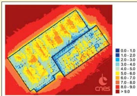
FIGURE 4 Average number of available A-GPS signals in acquisition mode
