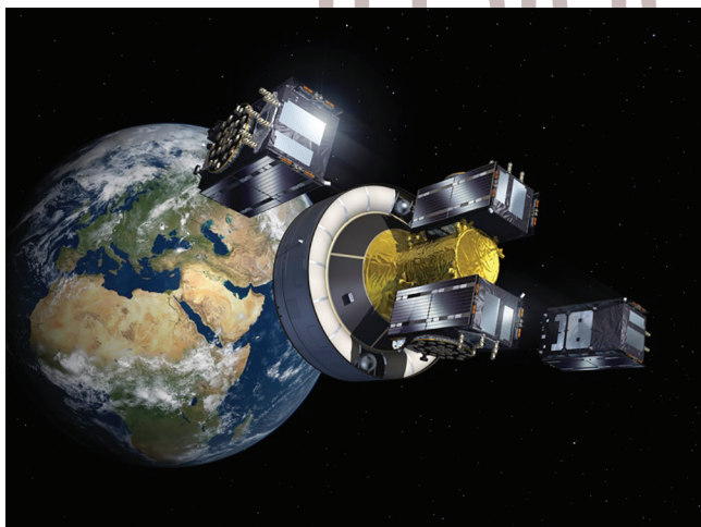
Galileo satellites 15–18 being deployed from their dispenser; they deploy two at a time, with the second pair deploying 20 minutes after the first. ESA
