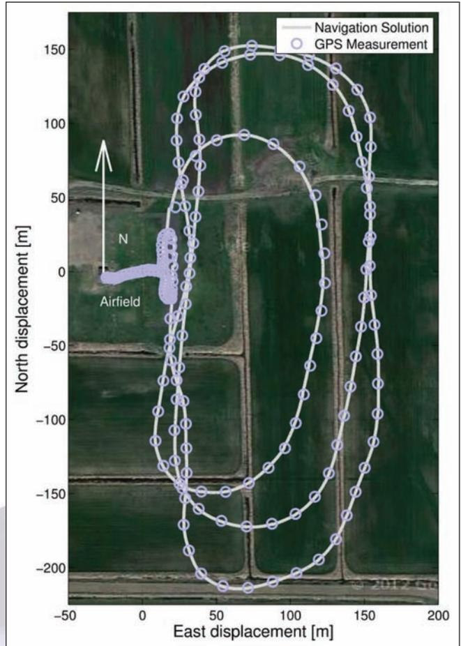
FIGURE 6 Navigation solution from INS/GPS integration algorithm
