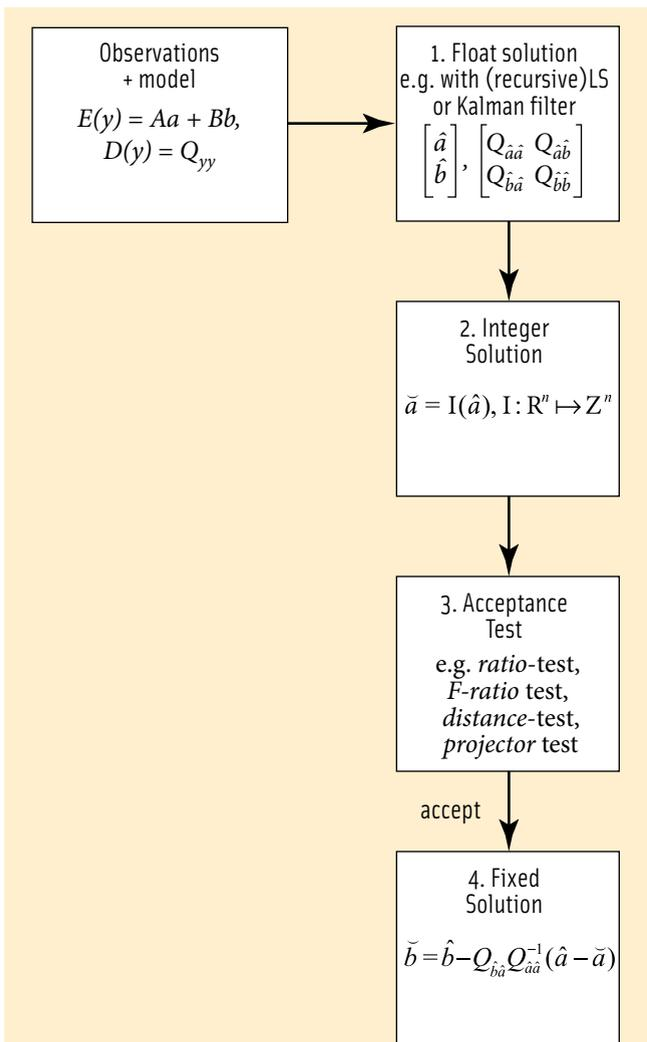
FIGURE 1 The four steps of GNSS carrier-phase ambiguity resolution
