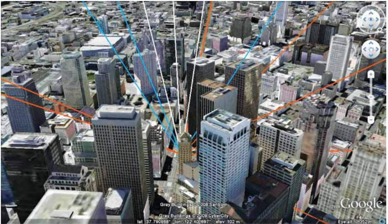
FIGURE 8 Satellite signals in San Francisco field trial: orange = blocked-but-reflected signals, white = LOS GLONASS, and blue = LOS GPS
