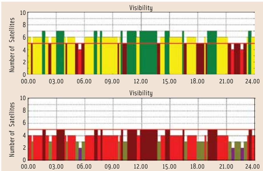
FIGURE 2 Simulated test results for San Francisco showing satellite visibility with a GPS-only receiver (bottom graph) and GPS plus SBAS (top graph)
