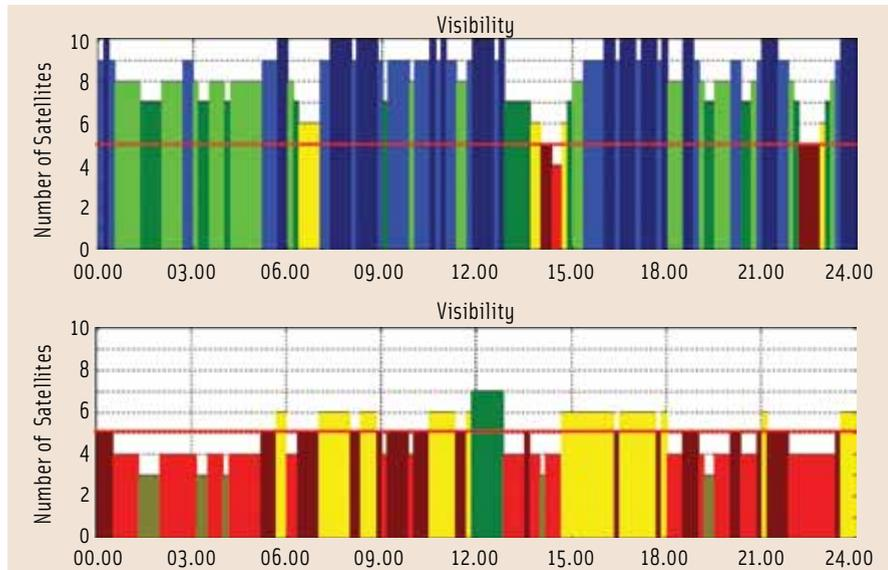
FIGURE 6 Simulated test results for Madrid showing satellite visibility with a GPS-only receiver (bottom graph) and GPS plus GLONASS (top graph)
