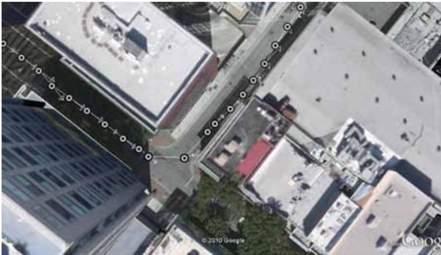
FIGURE 13 Detail from Figure 12, Lighston Alley, less than five meters wide. As can clearly be seen, multi-GNSS accuracy is good to a few meters, even in this environment.
