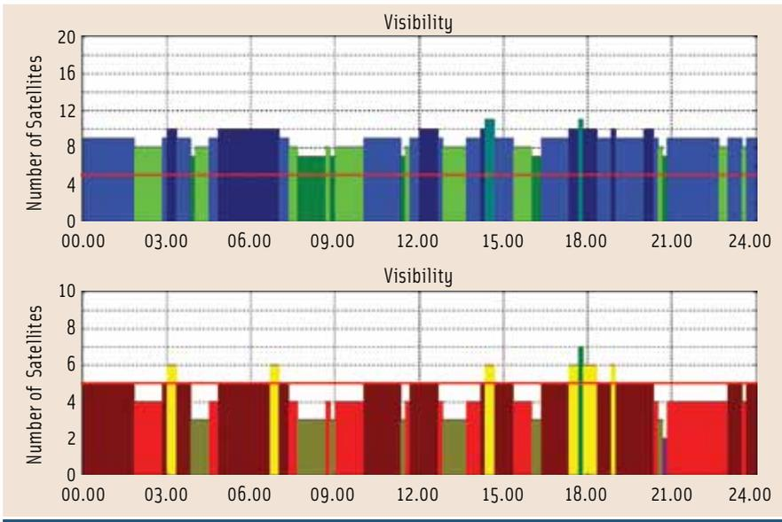
FIGURE 4 Satellite visibility in simulated Tokyo test with a GPS-only receiver (bottom graph) and GPS plus SBAS and QZSS (top graph)
