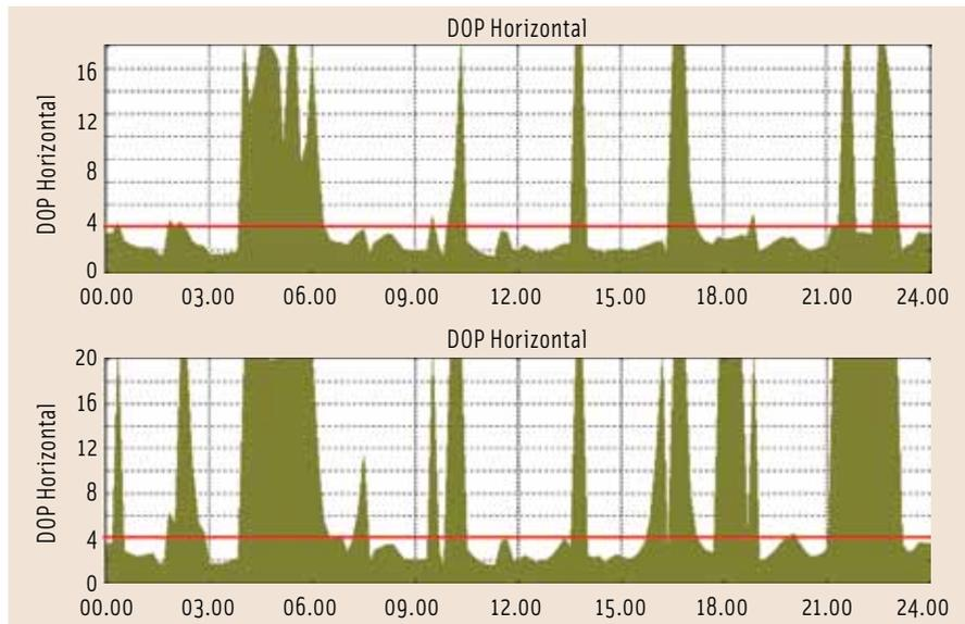
FIGURE 3 HDOP values in simulated San Francisco test with a GPS-only receiver (bottom graph) and GPS plus SBAS (top graph)
