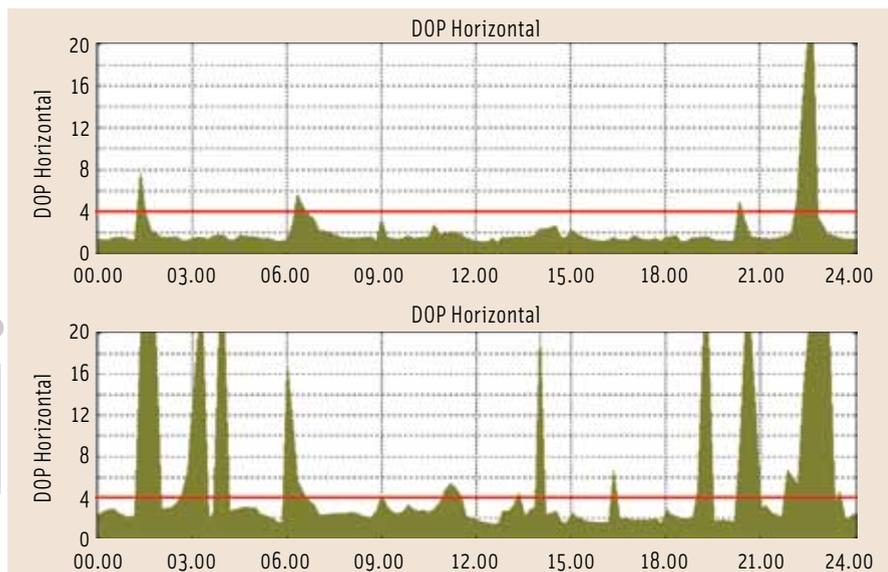
FIGURE 7 HDOP values in simulated Madrid test with a GPS-only receiver (bottom graph) and GPS+GLONASS plus SBAS (top graph)
