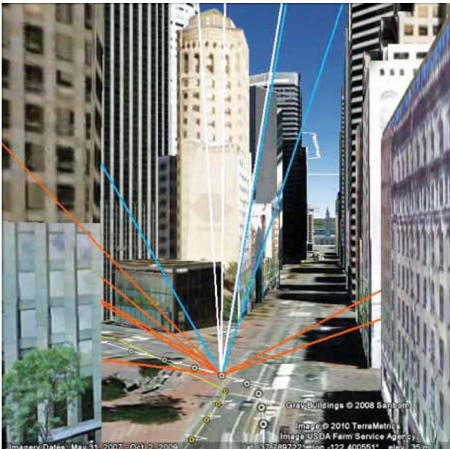
FIGURE 9 Satellite signals at street level in San Francisco field trial: orange = blocked-but-reflected signals, white = LOS GLONASS, and blue = LOS GPS
