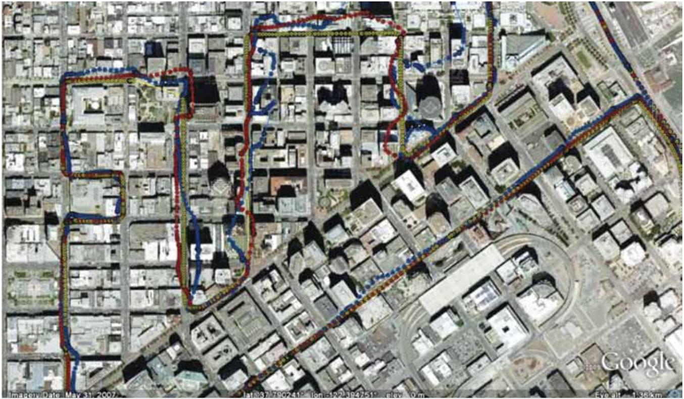
FIGURE 10 Test drive in San Francisco financial district. Colored lines show vehicle tracks as recorded by the following: yellow, truth data collected by the GNSS/IMU system; blue, results from GNSS/SBAS/BT/FM receiver with GLONASS disabled; red, receiver results with GPS+GLONASS.
