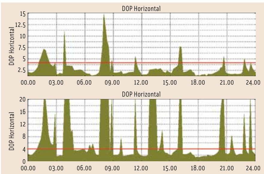
FIGURE 5 HDOP values in simulated Tokyo test with a GPS-only receiver (bottom graph) and GPS plus SBAS and QZSS (top graph)
