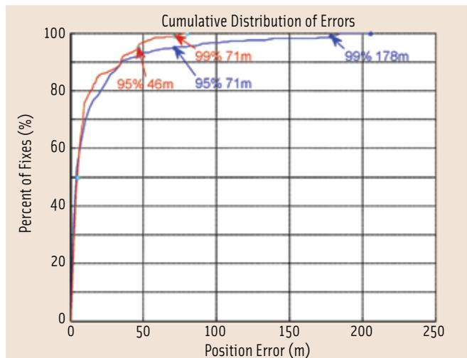
FIGURE 11 Comparison of GPS-only (blue line) and GPS+GLONASS (red line) cumulative distribution of errors in San Francisco driving test
