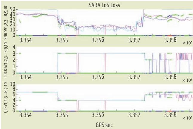
FIGURE 20 SNR and signal lock evolution by PRN during an LoS loss event
