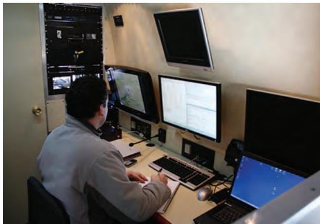
Inside view of the UAV ground control station
