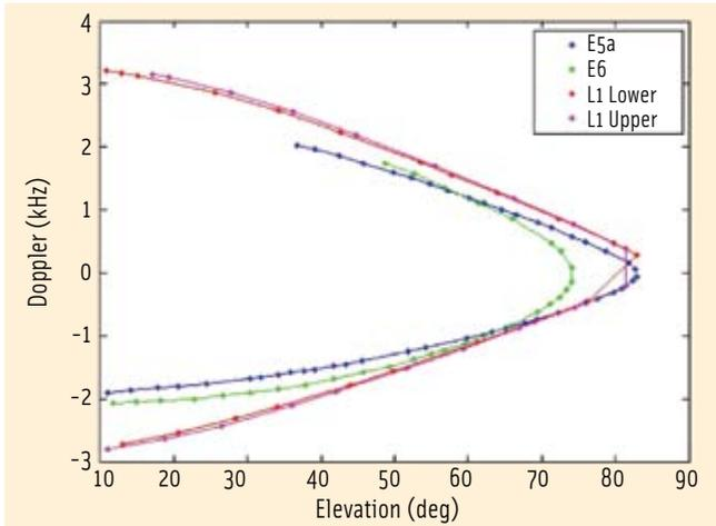
FIGURE 4 Measured Doppler on CW signals
