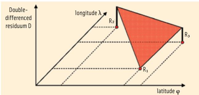
FIGURE 2 Illustration of the standard plane modeling method using northward and eastward gradients and three reference stations R1, 2, 3.
