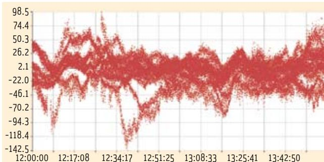
**FIGURE 1** Double difference ionospheric delays derived from dual frequency GPS data during typical (i.e. relatively calm) ionospheric conditions as currently observed in mid-latitudes; baselines: 56-78 km. (x-axis: GPS time hh:mm:ss; y-axis:  $\nabla\Delta ION$  in millimeters).
