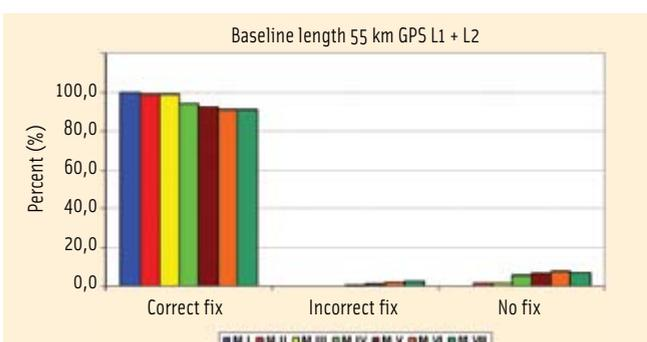
FIGURE 12 Network type "Thinned Out"; current GPS only configuration (L1 and L2); statistics of correct ambiguity fixing
