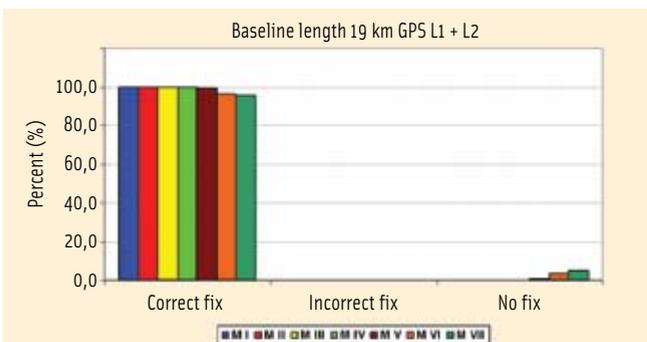
FIGURE 10 Network type "small"; current GPS only configuration (L1 and L2); statistics of correct ambiguity fixing
