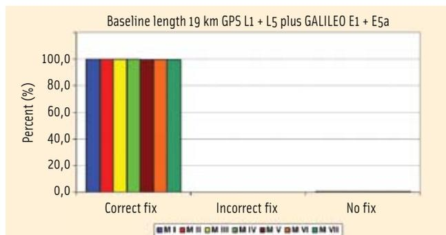
FIGURE 11 Network type "small"; dual frequency GPS and Galileo configuration; statistics of correct ambiguity fixing
