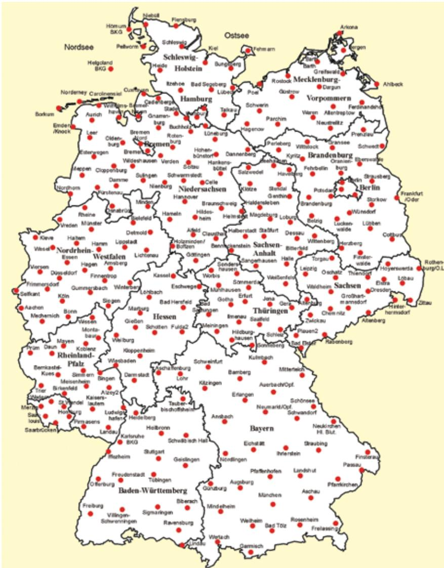
FIGURE 3 Stations of the German active reference station network (Each red dot indicates a reference station)
