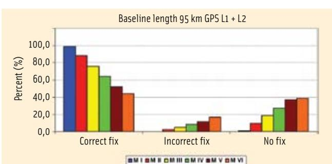
FIGURE 14 Network type "Challenging"; current GPS only configuration (L1 and L2); statistics of correct ambiguity fixing
