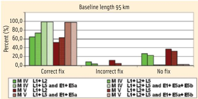
FIGURE 16 Network type “Challenging”; dual/triple frequency GPS and Galileo configurations; statistics of correct ambiguity fixing; only scenarios M IV and M V (strong ionospheric behavior)
