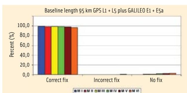
FIGURE 15 Network type "Challenging"; dual frequency GPS and Galileo configuration; statistics of correct ambiguity fixing
