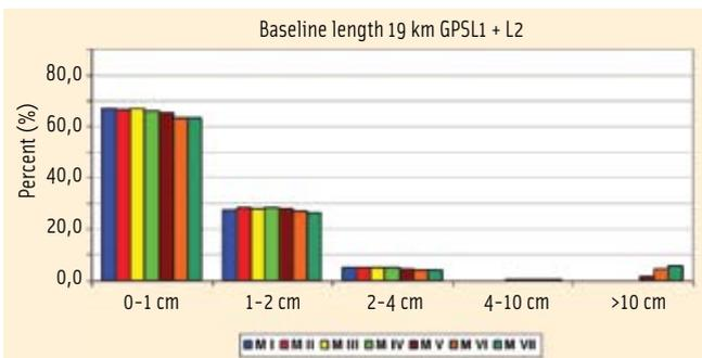
FIGURE 8 Network type "small"; current GPS-only configuration (L1 and L2); 3D position difference to nominal coordinates. See Table 2 for a description of the ionospheric parameters reflected in the legend.
