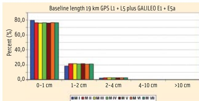
FIGURE 9 Network type "small"; dual frequency GPS and Galileo configuration; 3D position difference from nominal coordinates
