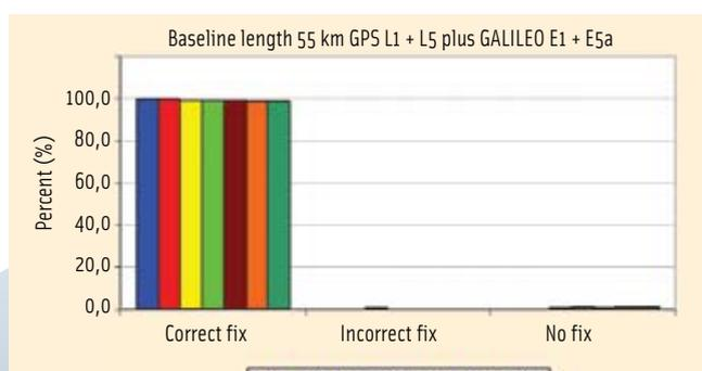
FIGURE 13 Network type "Thinned Out"; dual frequency GPS and Galileo configuration; statistics of correct ambiguity fixing.
