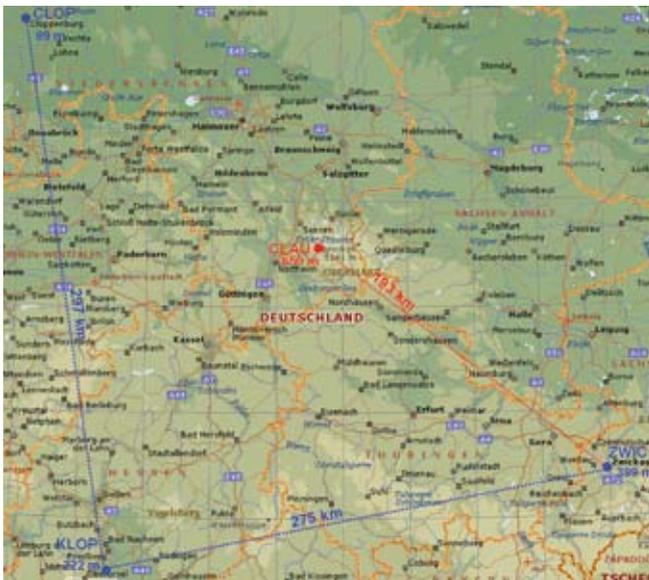
FIGURE 7 Type “Extreme”: Network triangle configuration with a baseline length of 193 kilometers to the nearest reference station.
