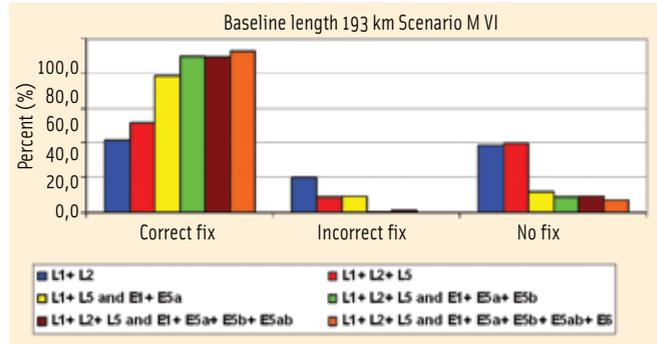
FIGURE 18 Network type “Extreme”; use of two/three/four/five frequencies GPS and GALILEO configuration; statistics of correct ambiguity fixing; only scenarios M VI (strong ionospheric behavior)
