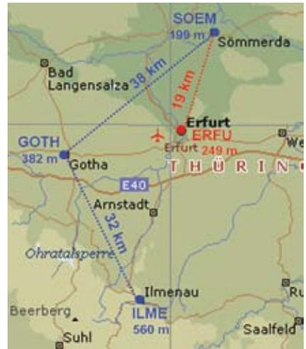
FIGURE 4 Type "Small": a typical Adv network triangle with a baseline length of 19 kilometers between rover and nearest reference station
