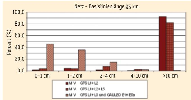
FIGURE 17 Network type “Challenging”; dual/triple frequency GPS and Galileo configuration; only scenario M V; 3D position difference to nominal coordinates
